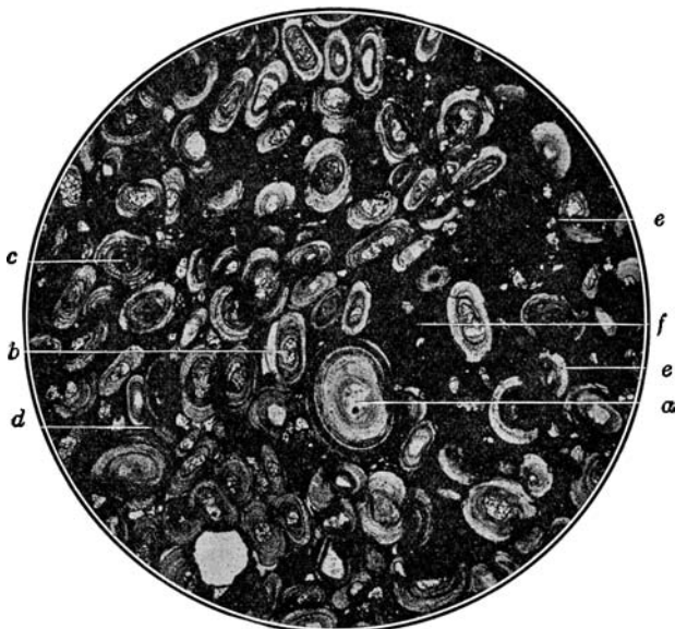
FIG. 110.—Ore from Silurian beds at La Ferrière-aux-Étangs, France. Magnified 22 diameters. The oörites are chlorite with a kernel of siderite; the fine-grained cement is chlorite and siderite. a , oörite of chlorite, in center of lighter color; partly converted into hematite on the outside; b , nucleus of corroded pure siderite; c , same of yellow, altered siderite; d , grains of siderite in the cement; e , chloritic oörite, partly crushed and invaded by cement; f , blackish cement of chlorite and siderite. (After L. Cayeux .)
