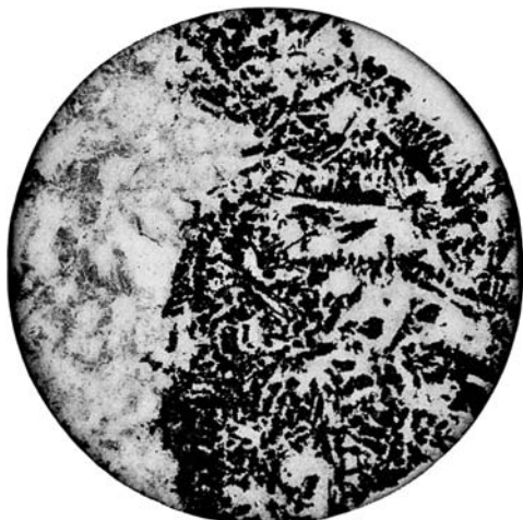
FIG. 184.—Dendritic gold (black) in extremely fine-grained quartz of probable colloidal deposition. White area is coarsely crystalline comb quartz, National, Nevada. Magnified 15 diameters.
