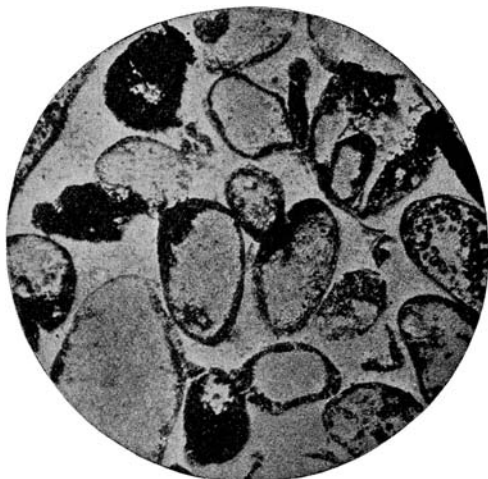
FIG. 121.—Ferruginous chert with greenalite granulites, in part replaced by ferric oxide (black). Magnified 40 diameters. (After C. K. Leith.)
