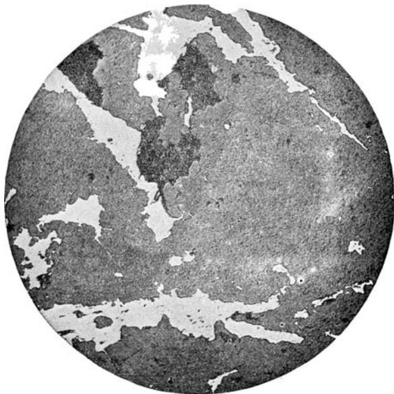
FIG. 58.—Replacement veinlets of galena (white) in cryptocrystalline quartz (dark gray) with vugs (black). Tintic, Utah. Magnified 11 diameters.
