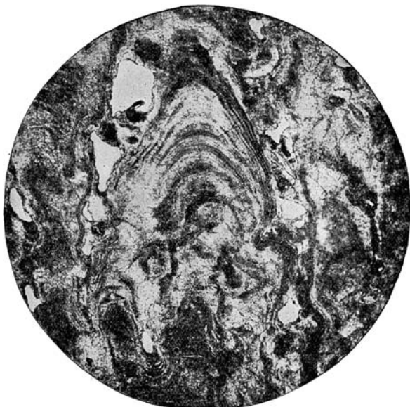
FIG. 7.—Section of opaline silica showing colloform structure. Yellowstone National Park. Magnified 32 diameters. (After H. C. Boydell, "Economic Geology.")
