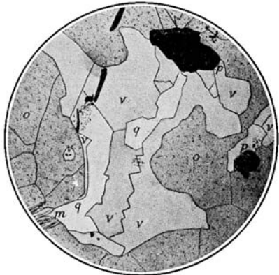
FIG. 190.—Filled space of dissolution in granite, Independence mine, Cripple Creek (granite ore). o , orthoclase of granite; m , biotite replaced by adularia and pyrite; v , adularia (secondary orthoclase), showing crustification; q , quartz; p , pyrite. Magnified 14 diameters.
