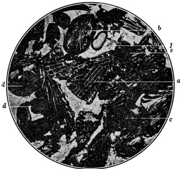
FIG. 108.—Clinton ore, Wolcott, Wayne County, New York. Magnified 20 diameters. Ore essentially formed of remains of bryozoans and crinoids. a , fragments of bryozoans, ferric oxide; b , fragment of bryozoan encrusted with ferric oxide; c , bryozoan structure almost obliterated by ferric oxide; d , crinoid stalk replaced by ferric oxide, cells filled with calcite of uniform optical orientation; e , same, almost entirely replaced; J , calcite cement. (After L. Cayeux.)
