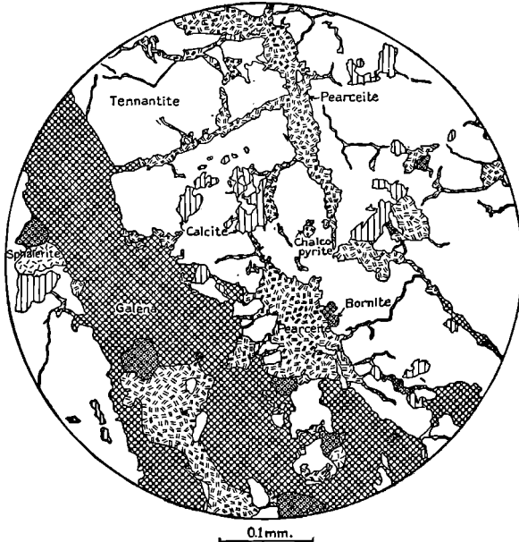
FIG. 241.—Tennantite traversed by late primary replacement veinlets of pearceite, base-metal sulphides, and calcite. Smuggler Hill workings, thirteenth level, Aspen, Colorado. Camera lucida drawing from polished specimen. (After E. S. Bastin, U. S. Geol. Survey.)
