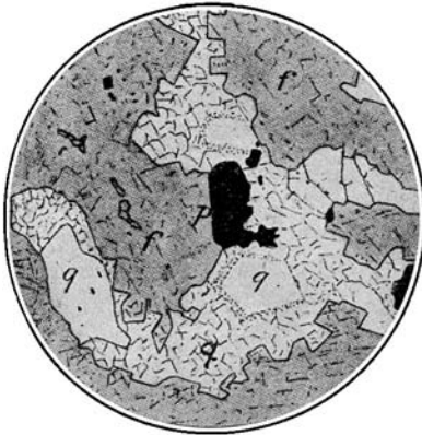
FIG. 189.—Vein filling, Portland mine, Cripple Creek (purple quartz). f , fluorite; q , quartz of coarser and finer grain; p , pyrite. Magnified 50 diameters.
