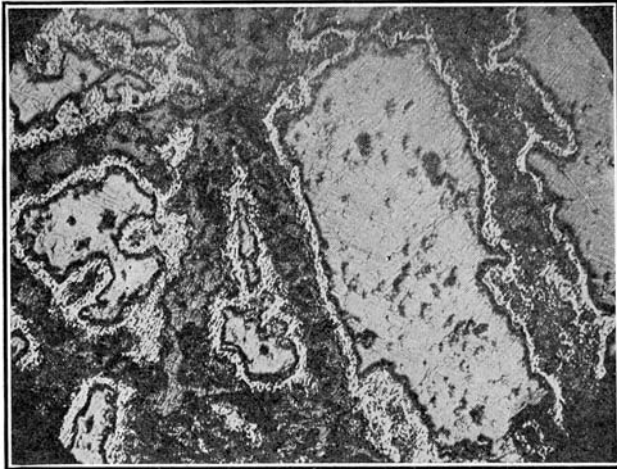
FIG. 70.—Polished section showing rims of argentite replacing sphalerite from the periphery. Crown King, Arizona. Magnified 90 diameters.
