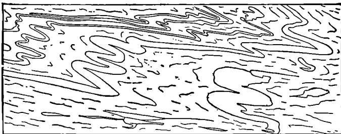
FIG. 19.—Gneiss with corrugated veinlets of quartz. (After C. R. Van Hise, U. S. Geol. Survey .)
