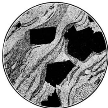
FIG. 165.—Crystals of galena developing in shaly dolomite. Black, galena; shaded and stippled, shaly dolomite; white, quartz. Magnified about 10 diameters. (After E. R. Buckley.)
