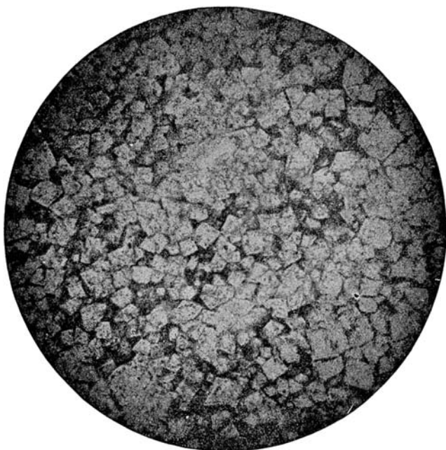
FIG. 61.—Thin section of dolomite completely silicified, but retaining texture and crystal form. (After J. D. Irving, U. S. Geol. Survey.)
