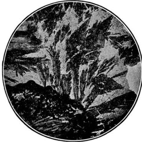
FIG. 317.—Photomicrograph of thin section showing azurite crystals replacing kaolin. Morenci, Arizona. Magnified 15 diameters.
