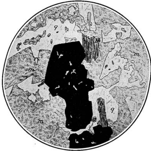
FIG. 209.—Altered granodiorite, Bellefountain mine, Nevada City, California. m , fine aggregate of sericite with some calcite and quartz, replacing orthoclase and andesine; b , original biotite altered to sericite; q , original quartz; black, pyrite with included sericite. Magnified 15 diameters.
