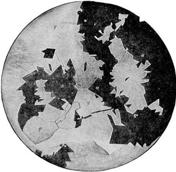
FIG. 167.—Intergrowth of quartz ( q ) and adularia ( a ), Fraction vein, Tonopah, Nevada. Magnified 38 diameters. (After J. E. Spurr, U. S. Geol. Survey. )
