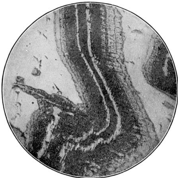
FIG. 315.—Polished section showing oxidation of enargite, Tintic, Utah. White, enargite; dark, copper arsenate; light gray, chalcocite. Magnified 360 diameters.
