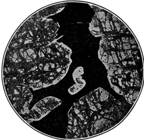
FIG. 308.—Thin section of olivine corroded by pyrrhotite and chalcopyrite, East Union, Maine. Magnified 15 diameters. (After E. S. Bastin.)
