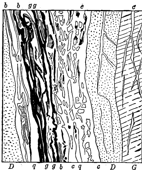
FIG. 233.—Section of the Adalbert vein at Przibram, Bohemia. G, graywacke; D, diorite; q, quartz; c, calcite; g, galena; b, sphalerite. (After J. Zadrazil and J. Schmidt.)
