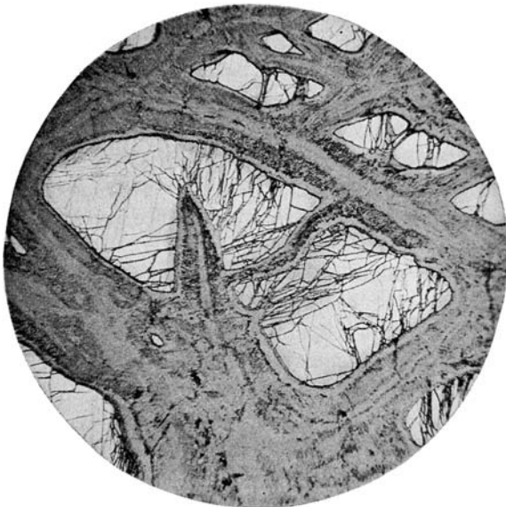
FIG. 320.—Supergene chalcocite (gray) replacing pyrite (white), Ray, Arizona. Magnified 120 diameters. (After L. C. Graton. )
