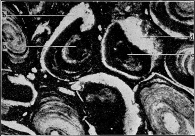
FIG. 111.—Oölitic chamosite-hematite ore of Wabana with siderite. a , spherule of hematite and chamosite in concentric layers; b , outer border of siderite, replacing spherule; c , spherule of hematite-chamosite partially replaced by siderite; d , siderite replacing spherule and matrix. Magnified 110 diameters. (After A. O. Hayes.)
