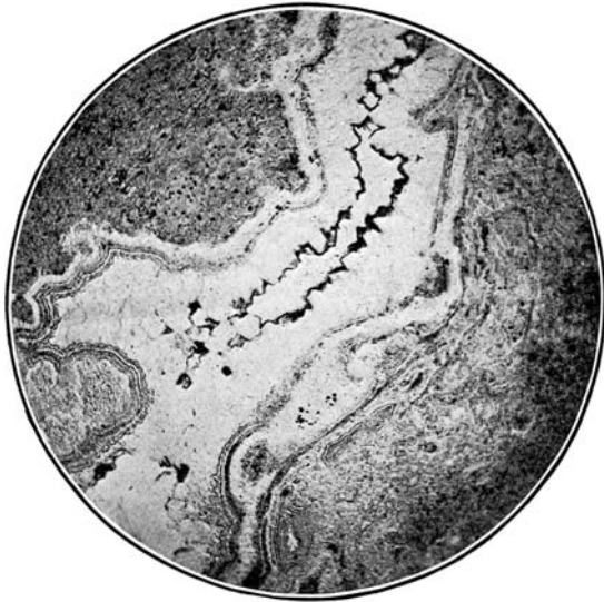
FIG. 5.—Section of chalcedonic spring deposits from Steamboat Springs, Nevada, showing colloform structure. White areas microcrystalline quartz. Magnified 25 diameters.
