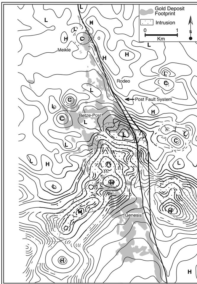
FIG. 13. Total magnetic intensity, reduced to pole for the Blue Star-Goldstrike subdistrict. Contour intervals 10 nt ( $\gamma$ ). Magnetic highs (H) and lows (L) are indicated. Magnetic highs due to mining infrastructure are designated by C. Footprints of gold deposits and intrusions are projected to surface. Magnetic contours by Pearson, deRidder and Johnson, Inc.
