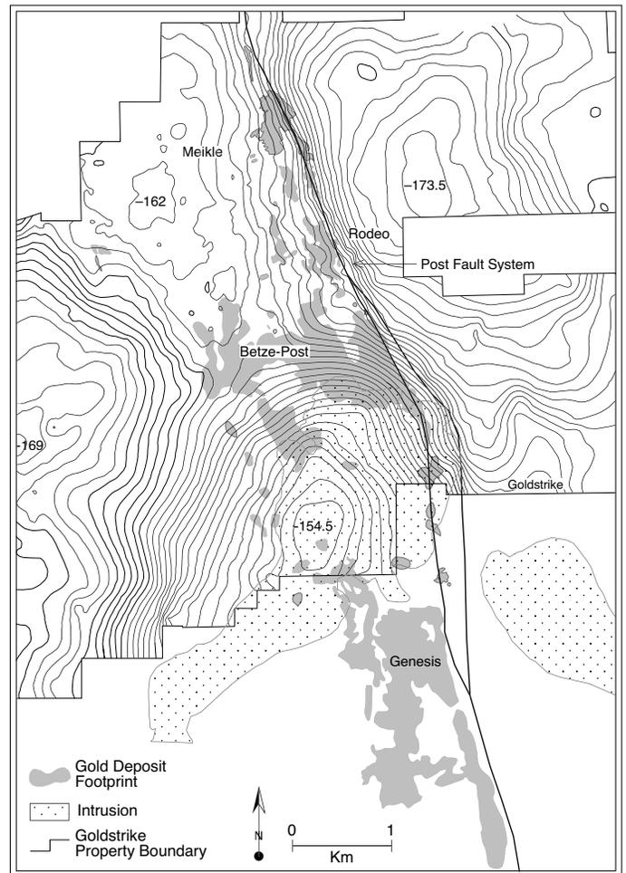
FIG. 14. Complete bouguer gravity for the Blue Star-Goldstrike subdistrict. Contour interval 0.5 mgal. Select highs and lows indicated. Footprints of gold deposits and intrusions are projected to surface. Gravity by Zonge Geosciences, Inc.
