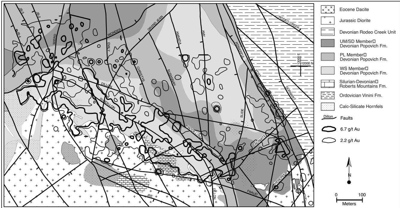
FIG. 9. Level plan at the 4700 level (1,433 m elevation) of the Betze and Deep Post subdeposits of the Betze-Post deposit. Important ore controls shown at this level are the Wispy Member of the Popovich Formation, the Dillon fault zone, and the contact of the Jurassic diorite. Small displacements on faults are not shown. The location of the level plan is shown in Figure 5.
