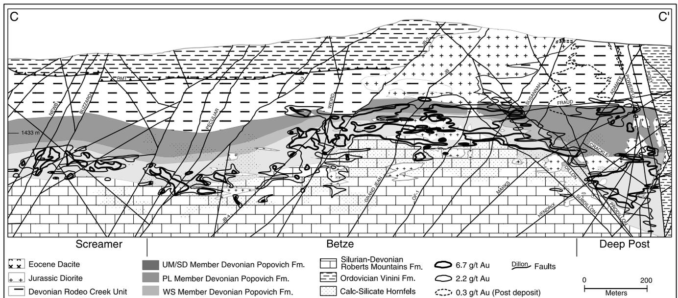
FIG. 8. Simplified east-west long section (C-C') of the Betze-Post deposit, showing the relationship of the orebodies to stratigraphic units and faults. The low-grade oxidized Post deposit is shown as a dashed outline. All other orebodies are unoxidized and refractory.
