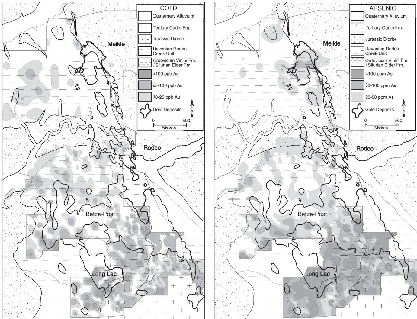
FIG. 12. Gold and arsenic soil geochemistry at Goldstrike, with simplified stratigraphic units, at surface. The outline of gold deposits is a projection to surface of orebodies at depths of 2 to 250 m. Only part of the area in the maps was sampled (boundary is indicated).
