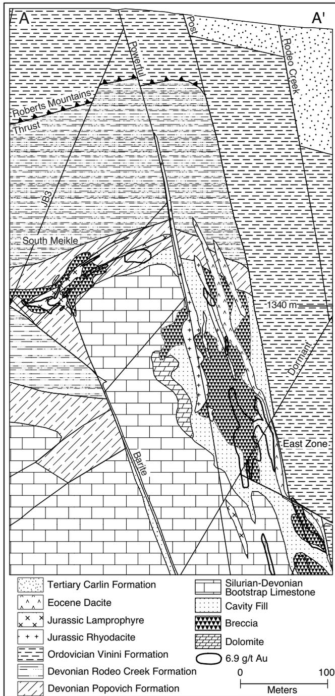
FIG. 10. Simplified cross section (A-A') of the Meikle and South Meikle deposits, showing the relationship of ore to breccias, intrusions, cavity-fill, and the Post fault zone. The East zone of the Meikle orebody is shown. The previously mined Upper Main zone at Meikle is located to the north of this section, above the East zone. Modified from Volk et al. (2000).
