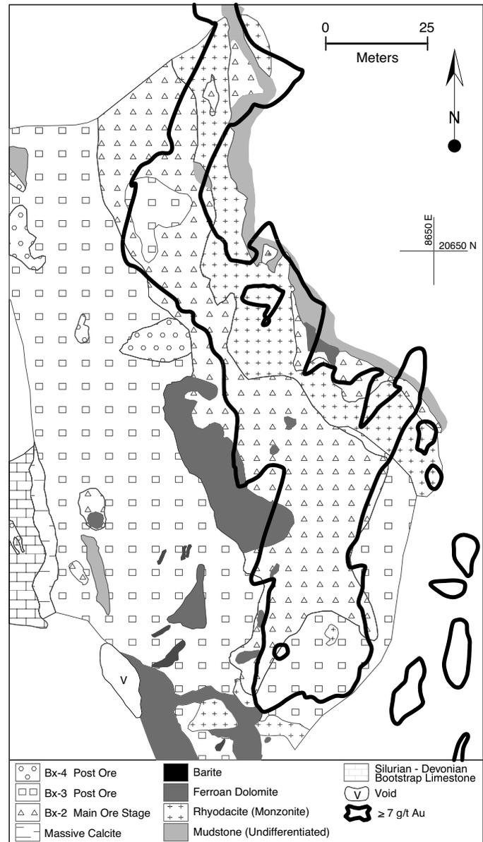
FIG. 6. Plan map of part of the 1375 level (1,294 m) elevation at the Meikle deposit, showing the orebody and the occurrence of breccia types, intrusions, dolomite alteration, and primary lithologies. Location of the level plan is shown in Figure 5. From Evans (2000).
