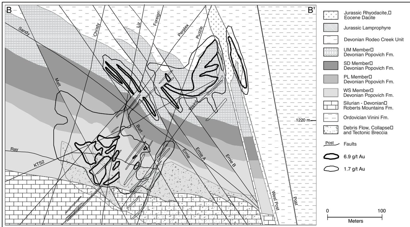
FIG. 11. Cross section of the Rodeo deposit (B-B'), showing the upper and lower ore zones in the Upper Mud and Wispy Members of the Popovich Formation. Structural ore controls include moderate to steep dipping faults that dip both east and west. Ground surface is at the 1,634-m elevation. Modified from Volk et al. (2000).
