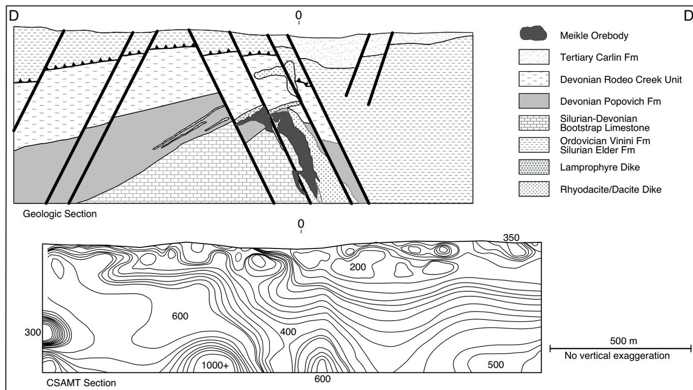
FIG. 15. Cross section D-D' across the Meikle deposit, showing geology and controlled source audio magnetotellurics (CSAMT) values in ohm-M. High-resistivity values correspond to the massive carbonate rocks of the Bootstrap limestone and low-resistivity values to the Carlin Formation. Geologic interpretation from drill holes prior to mining. Modified from Wright and Lide (1998).
