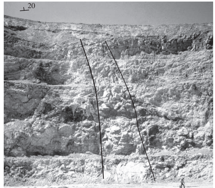
FIG. 13. Photograph, looking east, showing approximate outline of dike in the Rat deposit. Gold ore is concentrated along edges of the dike. Bedding of host lithology, shown at top of photograph, strikes about north and dips eastward at about 20^\circ . Benches are 40 ft in height. Photograph from Stephen G. Peters, USGS.
