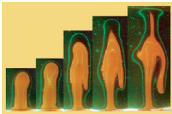
Figure 50 ‘Failing’ dome: A thermochemical dome was generated on a flat heater with a constant power. Initially the orange denser material was in a thin layer at the bottom of the tank. The green lines are the isotherms. Courtesy of Ichiro Kumagai and Kei Kurita.
