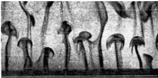
Figure 7 Thermal boundary layer instabilities in water visualized by an electrochemical technique. Adapted from Sparrow EM, Husar RB, and Goldstein RJ (1970). Observations and other characteristics of thermals. Journal of Fluid Mechanics 41: 793–800.
