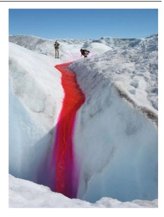
**Dye Tracer Investigations of Glacier Hydrology, Figure 1** Rhodamine dye flowing into a moulin during a tracer experiment on a glacier near the margin of the Greenland ice sheet.
