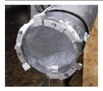
**Ice Core, Figure 1** Danish Hans Tausen Drill containing an ice core from Greenland from about 400 m depth. (Picture taken by Nancy Bertler.)
