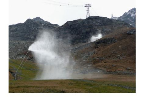
Artificial Production of Snow, Figure 2 Artificial snow production at temperatures above -3°C (Photo: Kees Woolthorn).
