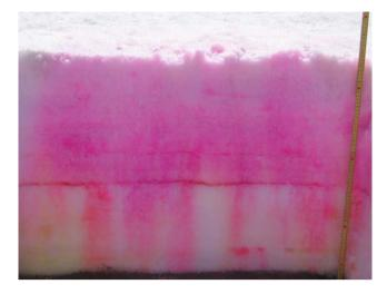
**Stratigraphy of Snowpacks, Figure 2** The pattern of percolation as revealed by dye-stained surface meltwater in an excavated snow-pit 2<sup>1</sup>/<sub>2</sub> h after a dye injection on the snowpack surface at Haut Glacier d'Arolla, Switzerland on 25 July 2004. An ice layer, 30 cm above the glacier surface, retains dye above it allowing continued downward flow through preferential flow-fingers. (Photo: F. Campbell).
