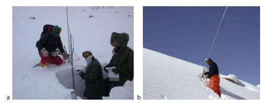
Snow Pit, Figure 1 Image (a) snow pit observation in progress, image (b) usage of Snow Micro Pen (SMP).
