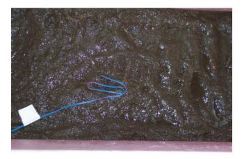
**Thermokarst, Figure 2** Preferential thaw settlement at room temperature after 5 h of thaw.
