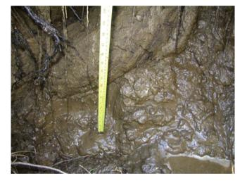
Thermokarst, Figure 5 Soil profile of the right bank eroding face of the gully demonstrating supersaturated soil conditions and slurry detachment from soil matrix under high fluid pressure. (Photograph taken on June 9, 2004 after a few days without any precipitation.)
