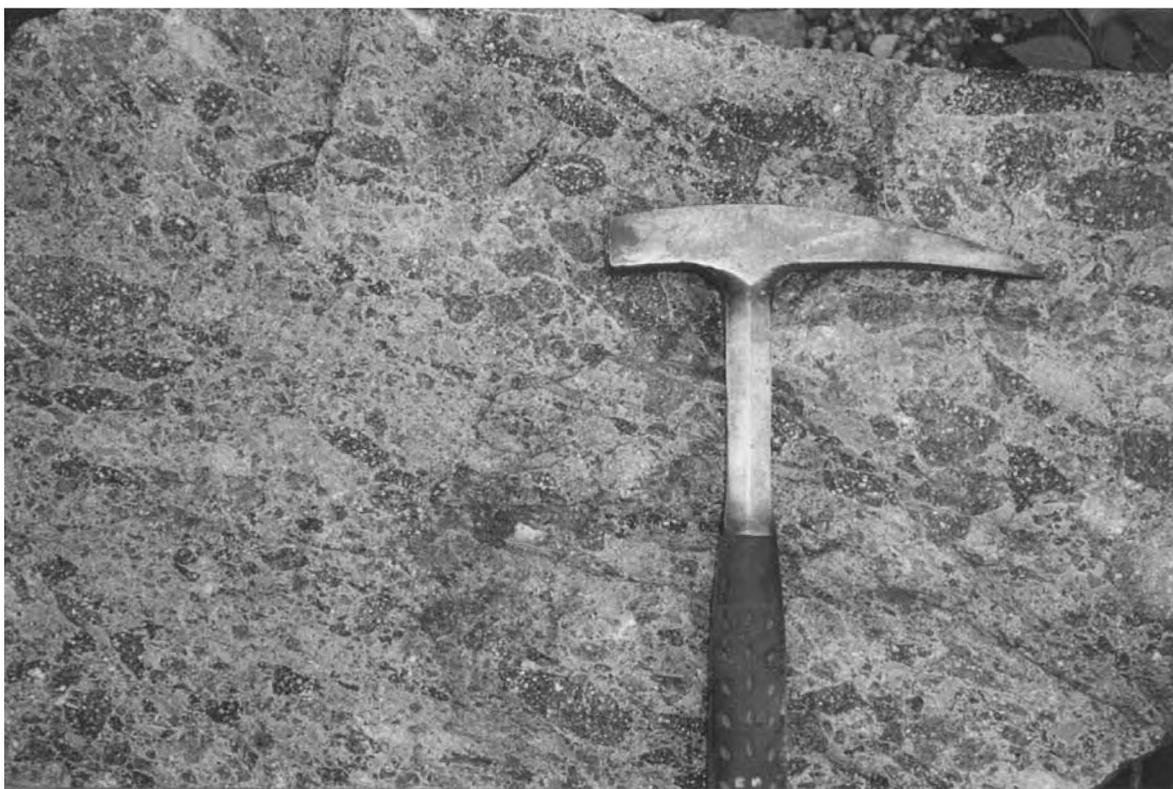
Fig. 3.12. Andesite tuff of Amut suite. Open-pit of Pereval'noe tin deposit
