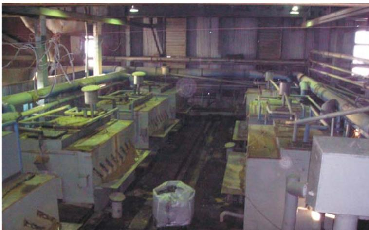
Fig. 4 CIP column type reactor – capacity 210 m<sup>3</sup> each (Kochkarsky gold plant, Ural)
