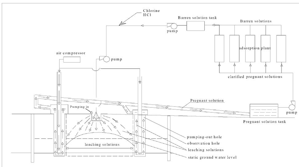
Fig. 6 In-Situ gold leaching process scheme
