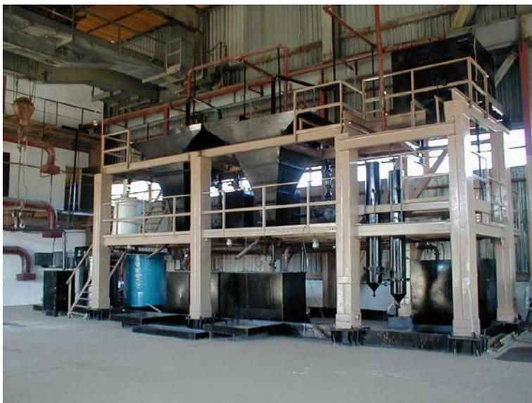
Fig. 2 Intensive cyanidation unit view
