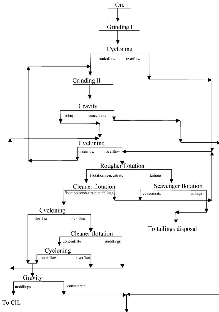
Fig. 5 Ore concentration flowsheet including flotation concentrate recleaning
