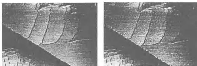
Figure 11. Atomic force micrographs illustrating complete crystal growth inhibition by PBTC on the (104) crystallographic face of calcite. The images obtained in situ are 2800 x 2800 nanometers with a vertical scale of 10 nanometers.
