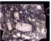
**Fig.** Diagnostic textures of HS epithermal deposits. (**1.**) Vuggy quartz caused by leaching of sanidine phenocrysts (≤4 cm long) by acidic fluid (pH <2 [55]). (**r.**) Same rock (quartz latite porphyry) altered to alunite-kaolinite in the alteration halo to vuggy quartz ore zone of Summitville deposit.
