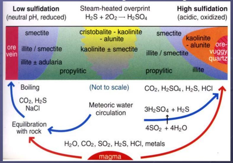
Quartz is stable throughout; propyllitic alteration occurs outside conduit zones (i.e., low water-rock ratio)
