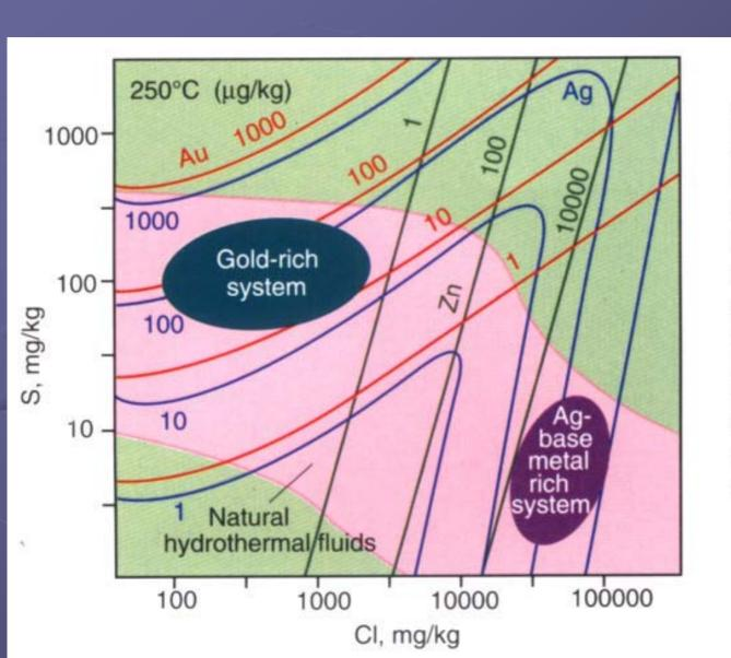
Fig. Solubility of Au, Ag, and Zn as a function of S and Cl concentration at pH and redox of LS mineral assemblages [24]. Clpoor solutions typical of Au-rich LS ore deposits [19] transport Au as bisulfide complexes, but cannot transport much chloride-complexed base metals [24].
