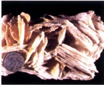
**Fig.** Banded botryoidal quartz vein from the Sleeper LS deposit, Nevada [44]; note electrum bands and quartz after bladed calcite (photo by J. Saunders). (**r.**) Coarse bladed calcite from the Martha Hill LS deposit, New Zealand (photo by S. Simmons).
