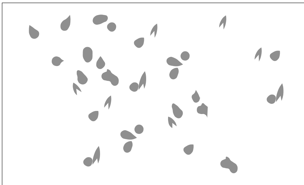
Figure 2 Alpha particle tracks visible in etched CR-39 (x 400)
