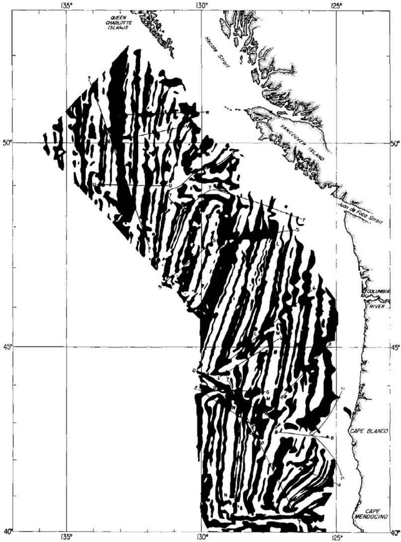
FIGURE 11.3 The celebrated index anomaly map of the total magnetic field produced by Raff and Mason. To uncover this spectacular pattern of anomalies, Mason reduced a vast amount of data acquired by a towed fluxgate magnetometer employed on many cruises. The total area surveyed was about 590,000 km 2 .
