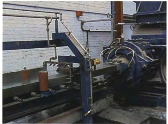
PLATE 17. Extruding of clay body for facing bricks. Hanson Brick, Kings Dyke, Peterborough, UK.
