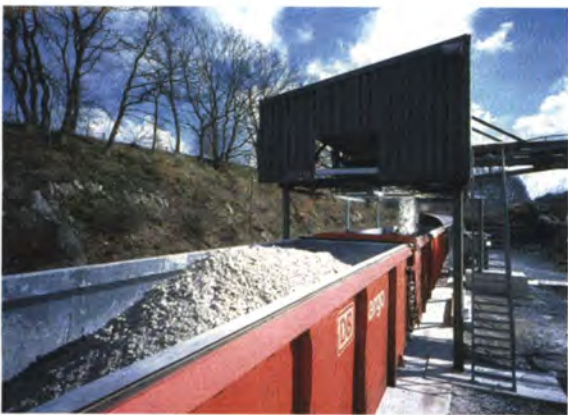
PLATE 22. Loading railway wagons with blended ball clay. WBB Fuchs GmbH, Westerwald region, western Germany.
