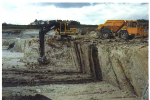
PLATE 19. Ball clay extraction, WBB Minerals Westbeare Quarry, Petrockstowe Basin, Devon. The dark seams are interbedded lignites.
