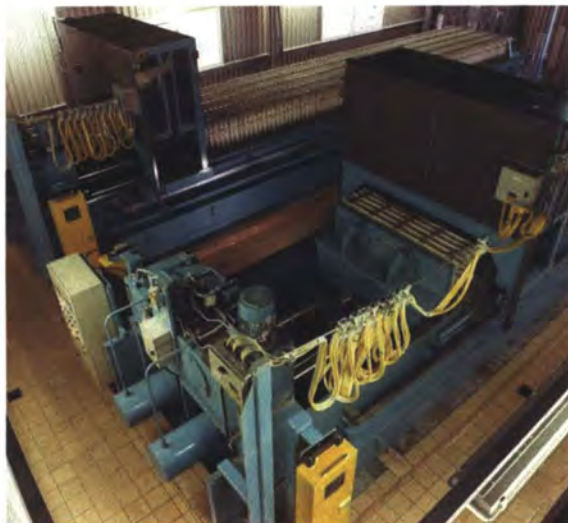
PLATE 25. Filter presses remove the water from the thickened kaolin slurry and create a kaolin filter-cake. WBB Minerals Cornwood processing plant, south-west Dartmoor, Devon, UK.
