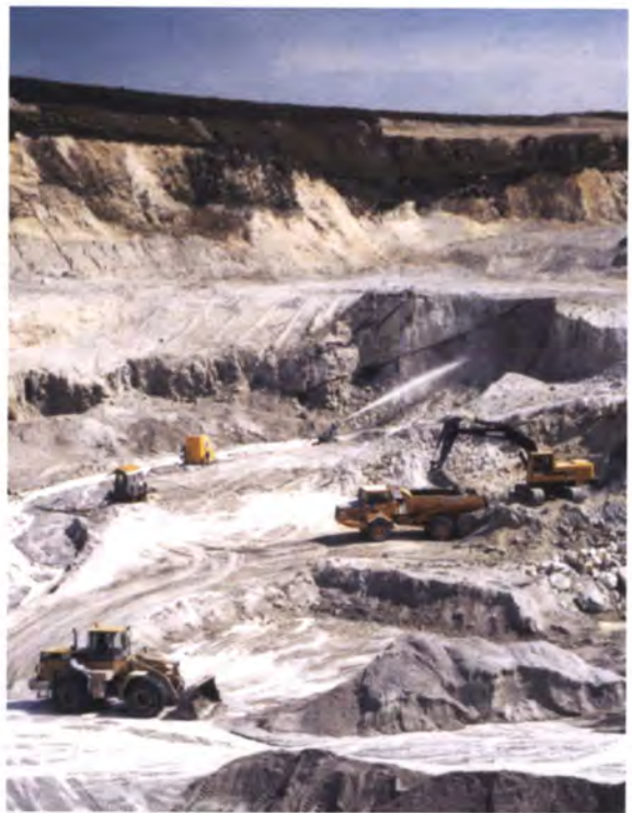
PLATE 23. Hydraulic mining of kaolinized granite (growan) using a high-pressure water monitor. The figure also shows the clearing of waste rock material (stent). WBB Minerals Headon Quarry, south-west Dartmoor, Devon, UK.
