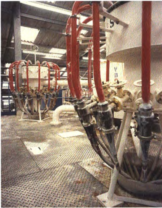
PLATE 24. Hydrocyclones are used to separate out the fine (kaolin) fraction from the growan (kaolinized granite) slurry. WBB Minerals Cornwood processing plant, Devon, UK.
