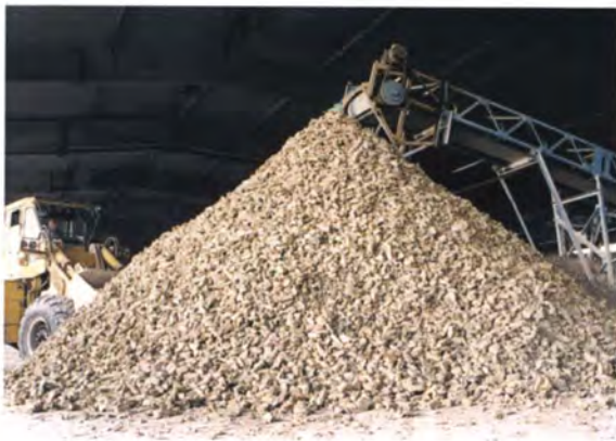
PLATE 21. Clay shredding to create a homogenised, ball clay blend. Donbas Clays JSC, Mertsalovo, Donbas region, eastern Ukraine.
