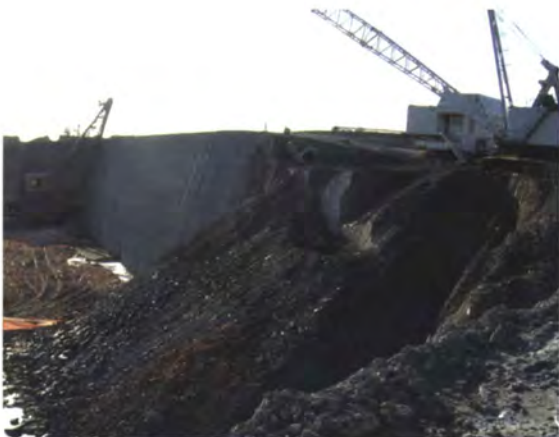
PLATE 16. Extraction of brick clays by shale planer and dragline. Hanson Brick, Kings Dyke West Quarry, Peterborough, UK.
