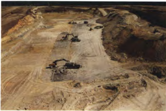
PLATE 20. Ball clay extraction in Donbas Clays JSC South October (southern) quarry, Donbas Region, eastern Ukraine. Quarry is advancing to left, and being backfilled on the right.
