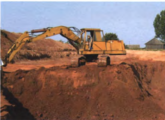
PLATE 15. Extraction of red clay for use in the brick industry. Hanson Brick, Torun, Poland.
