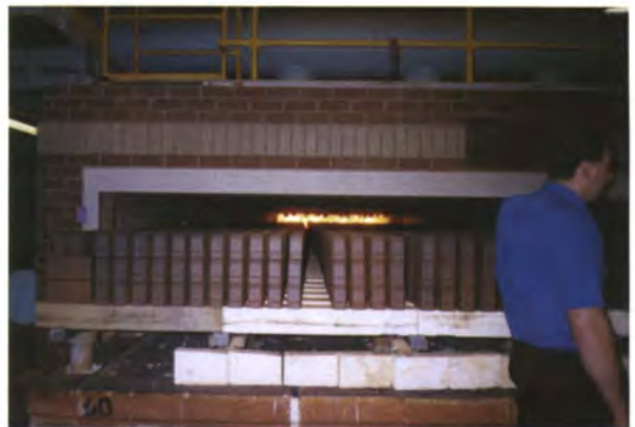
PLATE 18. Firing bricks in tunnel kiln. Hanson Brick, Pine Hall kiln, USA.
