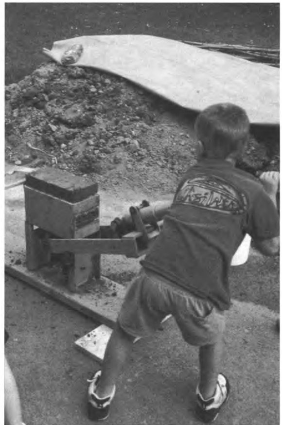
FIG. 13.5. Compressed blocks being manufactured at University of Plymouth.
