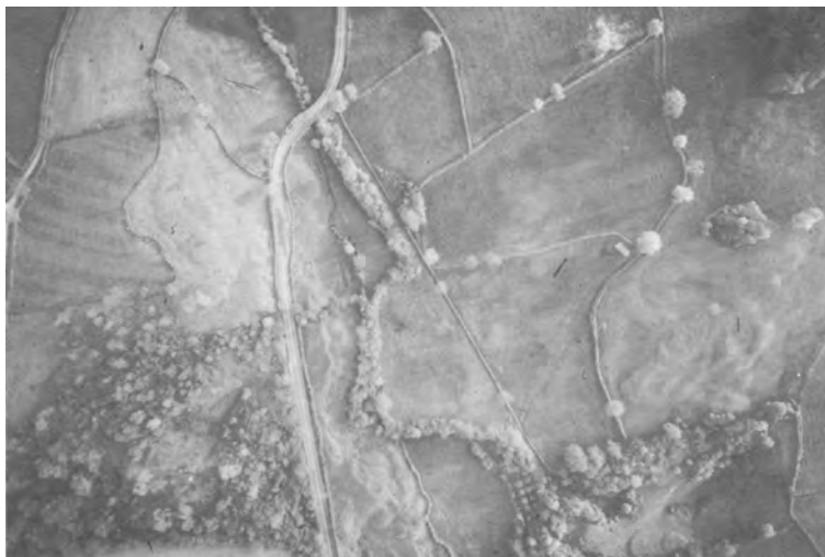
FIG. 7.4. Air photo showing clay terrain.
