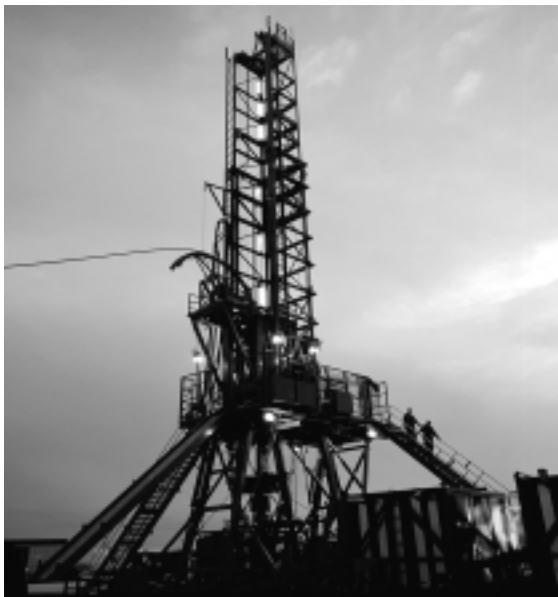
Figure 2-14 Galileo Coiled Tubing Drilling Unit
