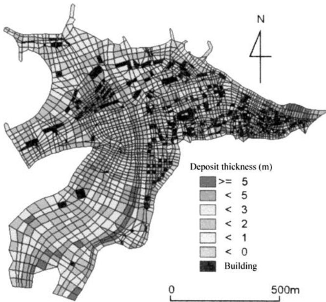
Figure 7.52 Distribution of deposit thickness obtained by reading aerial photographs.
