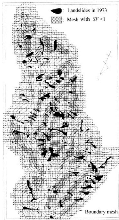
Figure 8.59 Existing landslides and the meshes experienced SF < 1 in 1971 rainfall in the Takoradani basin.
