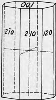
FIG. 141. Ditetragonal prism and base.
