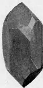
FIG. 210. Photograph of prism ( 10\bar{1}0 ), two rhombohedrons ( 10\bar{1}1 ) ( 01\bar{1}1 ), right trigonal pyramid ( 11\bar{2}1 ), and right trapezohedron ( 51\bar{6}1 ).
