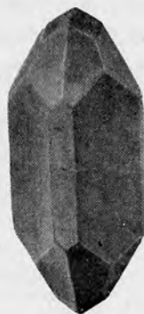
FIG. 147. Photograph of first and second order prisms, first order pyramid and ditetragonal dipyramid.
