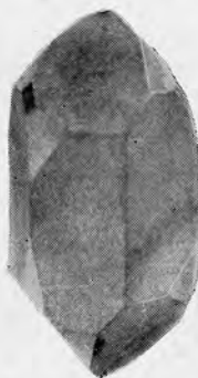
FIG. 212. Photograph of prism ( 10\bar{1}0 ), two rhombohedrons ( 10\bar{1}1 ) ( 01\bar{1}1 ), left trigonal dipyramid ( 2\bar{1}11 ), and left trapezohedron ( 6\bar{1}51 ).
