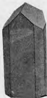
FIG. 201. Photograph of second order hexagonal prism ( 11\bar{2}0 ), trigonal prism ( 10\bar{1}0 ), two trigonal pyramids, ( 02\bar{2}1 ) and ( 01\bar{1}1 ) and base ( 000\bar{1} ).
