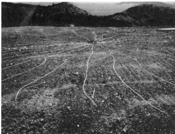
Fig. 33-13. Zortman, Little Rocky Mountains, Montana. Heap-leaching of blasted (but not crushed) rock made possible a profitable gold recovery from very low-grade auriferous stockworks and veins in syenite and quartz monzonite.
