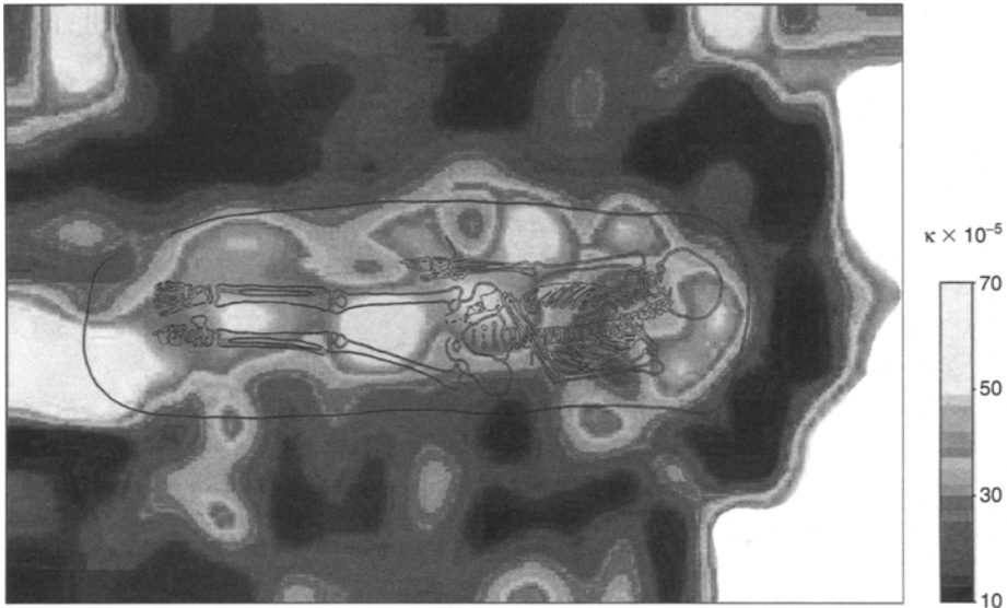
Figure 11.2 Magnetic susceptibility values recorded over an Anglo-Saxon grave at Lakenheath, England ( 0.6^{\circ}\text{E} , 52.4^{\circ}\text{N} ). The subsequently excavated skeletal remains are indicated. The color scale represents SI susceptibility ( \kappa ) values ranging from 10 \times 10^{-5} (black) to 70 \times 10^{-5} (white). The area shown measures 1.4 \times 2.1 m. The data were collected under the auspices of English Heritage using a Bartington MS2 meter (see Chapter 4). (Figure kindly provided by Neil Linford.) See color plate.
