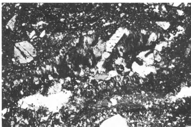
FIG. 5. The same photomicrograph as Fig. 4, showing the composite structure of the fiammé, which is made up of an outer zone of devitrified glass and an inner lighter one of slightly coarser quartzo-feldspathic mosaic. C.N. X35.
