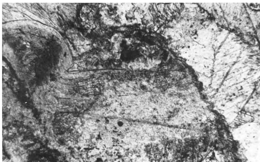
FIG. 11. Banding in chloritized amphibole flakes. Crossed nicols, \times 140 .
