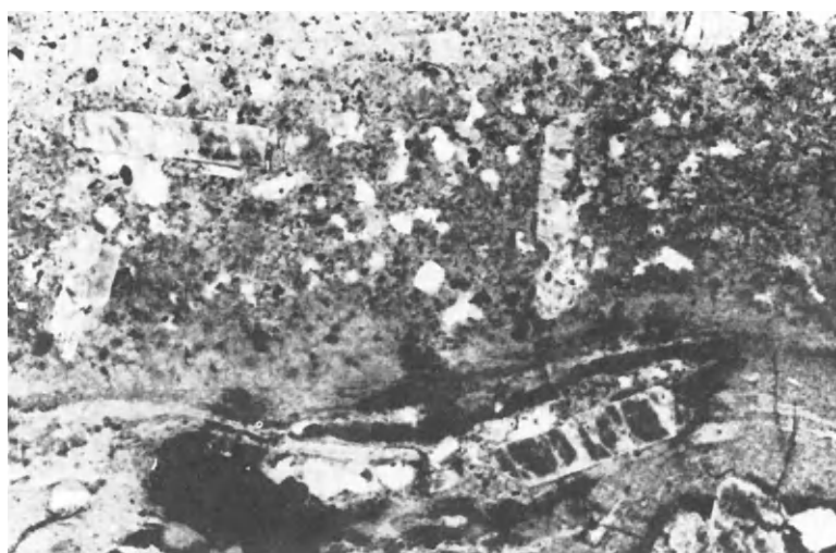
FIG. 6. Loosely welded tuff showing some of the feldspar crystals standing with their long axes at right angle to the lamination of the tuff as if they had fallen into it from above. P.L. X35.
