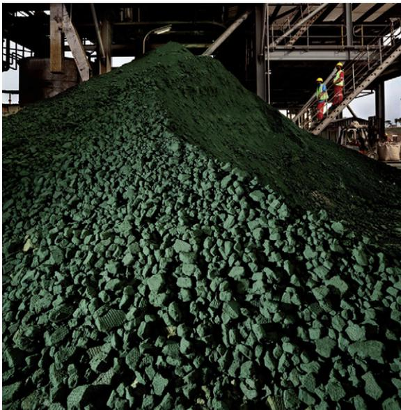
**FIGURE 30.6** Cobalt hydroxide produced from weathered copper–cobalt ore from Democratic Republic of Congo. It is sent to market for chemical production or redissolution and cobalt electroplating.
