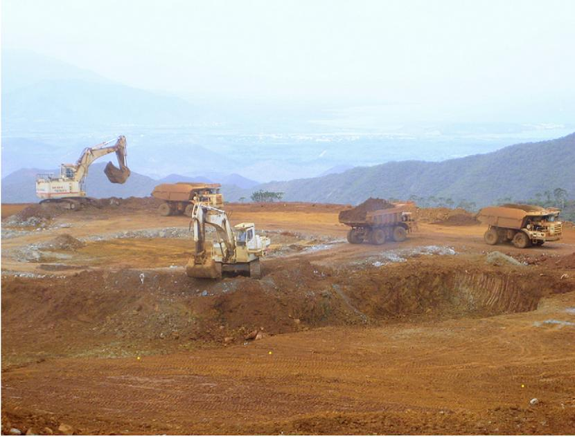
**FIGURE 1.2** Hill-top laterite mine in New Caledonia. The overburden has been removed to expose the saprolite ore, which is mined as shown, upgraded and smelted to ferronickel. The ore delivered to the process plant typically contains about 2% Ni. *Photograph courtesy W.G. Davenport.*
