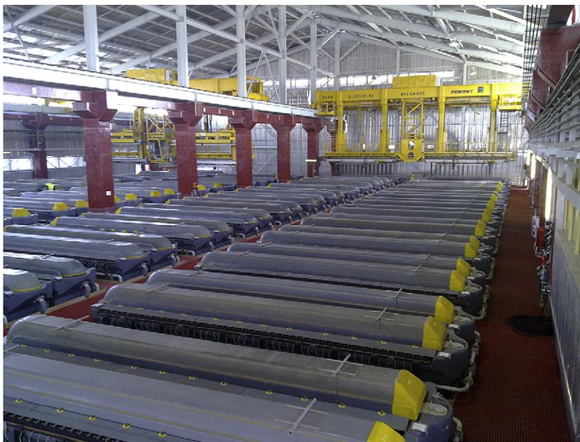
**FIGURE 26.5** The nickel tankhouse at Anglo American Platinum, showing the mist abatement hoods and the crane for automatic harvesting of the nickel cathodes. *Source: Photograph by J. J. Taute, courtesy of Anglo American Platinum*
