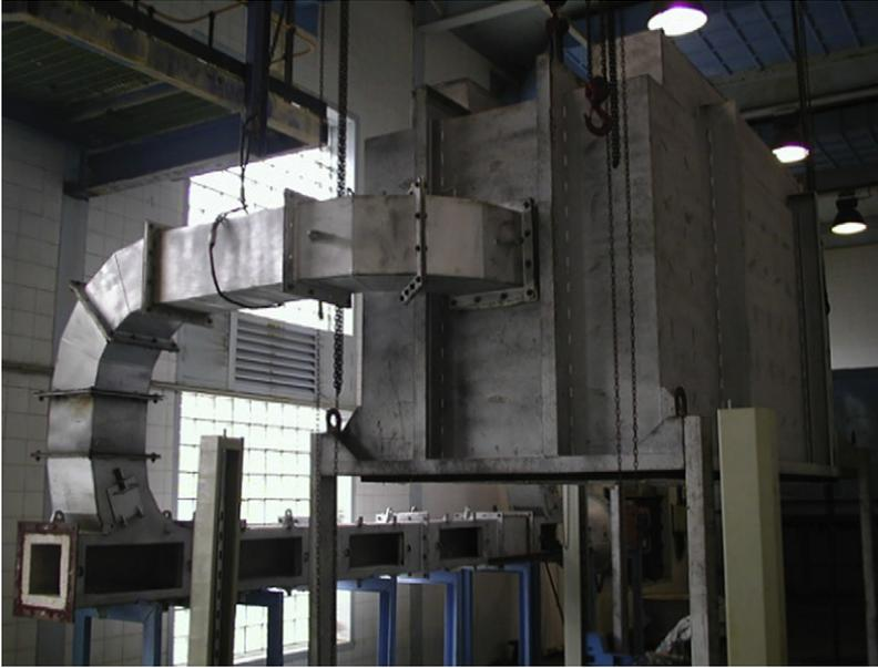
**FIGURE 37.4** An ignition furnace at Impala Platinum. Note the off-take ducting on the left-hand side of the furnace for the extraction of gases.
