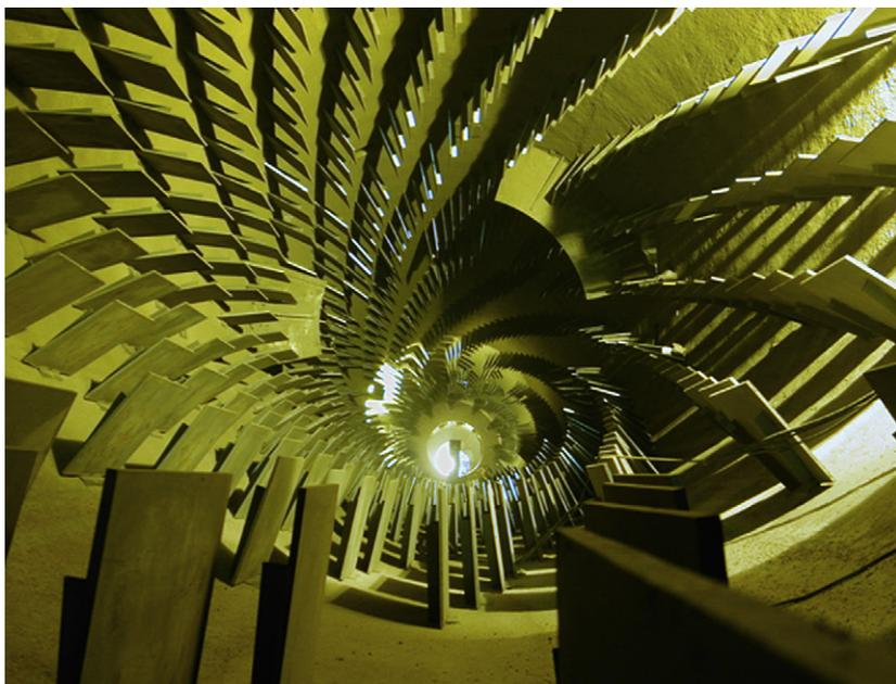
**FIGURE 5.1** Inside a new rotary calcination kiln. The internal lifters are notable. This kiln is 6 m diameter and 130 m long. It removes water from the partially dried feed and partially reduces nickel oxide to nickel metal. *Photograph courtesy of Hatch.*
