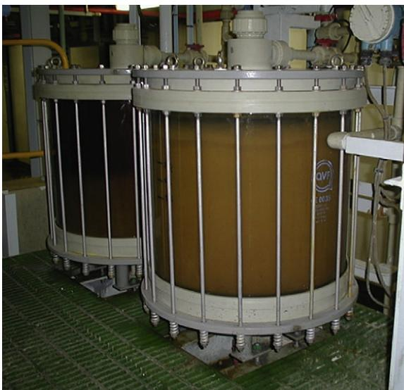
**FIGURE 37.13** The ion-exchange columns used for extracting palladium from solution containing, platinum, palladium, rhodium, iridium, ruthenium, osmium and base metals, such as copper, iron and nickel. The columns are loaded with SuperLig 2, which is highly selective for palladium. The columns are small in size because the kinetics of extraction are fast. *Photograph courtesy of Impala Platinum.*
