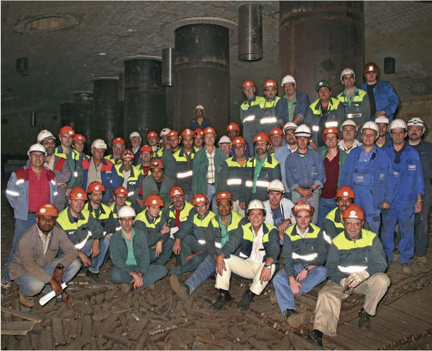
**FIGURE 6.1** Inside of refurbished laterite-to-ferronickel smelting furnace. Six suspended carbon electrodes, inside their steel ‘cans’, are shown behind the group. Each electrode has a diameter of 1.4 m. Calcine feed pipes can be seen between the electrodes. Note the scrap ferronickel on the floor. It is used to start up the furnace. *Photograph courtesy of Société Le Nickel-SLN/Eramet.*
