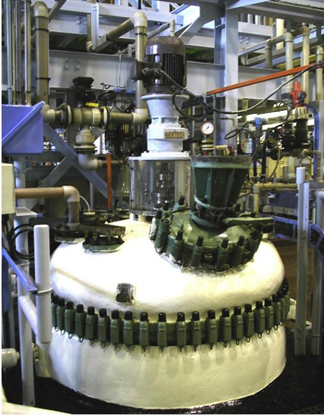
**FIGURE 37.1** A Grade 2 titanium vessel used for the dissolution of a PGM concentrate. The vessel has a volume of about 2.2 m<sup>3</sup>. The vessel is agitated and has a heating/cooling jacket. Chlorine is intermittently passed through the contents. *Photograph courtesy of Impala Platinum.*
