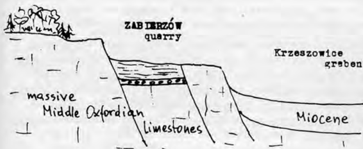
Fig. 86 Schematic section through the southern margin of the Krzeszowice graben, to show location of the Upper Cretaceous deposits within a small step-faulted graben exposed in the Zabierzów quarry ( cf. Fig. 77 - area indicated by an arrow)
