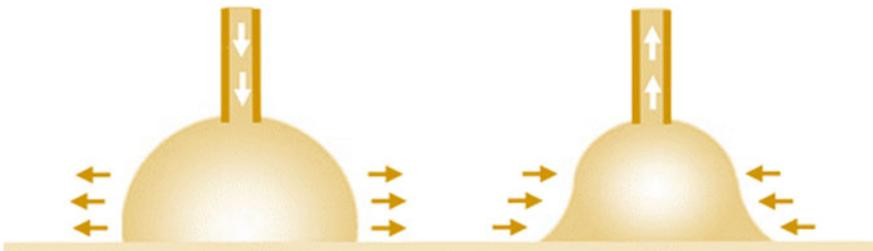
**Fig. 4.3** Diagram showing advancing and receding contact angles
