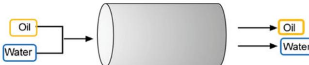
**Fig. 6.2** Schematic of unsteady-state and steady-state techniques of determining oil and water relative permeability
