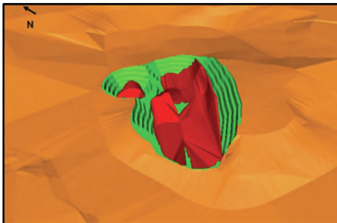
FIGURE 7.13 View of the geological model exposed on the surface with conceptual benches.
