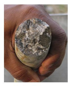
FIGURE 4.23 Photograph of drill core (Norite) cutting across the mafic and ultramafic layered igneous intrusive complex, being explored for chromium and platinum group of minerals at Boula-Nausahi, Orissa, India.
