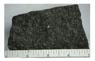
FIGURE 4.19 Dolerite is a medium-grained mafic intrusive igneous rock composed primarily of plagioclase set in a finer matrix of clinopyroxene ± olivine, magnetite and ilmenite. Source: Prof. Arijit Ray.
