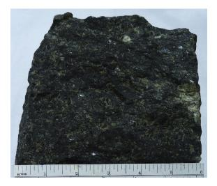
FIGURE 4.17 Gabbro is dark gray to greenish black color plutonic rock and chemically equivalent to volcanic basalt. The rock mainly contains Ca—plagioclase and ferromagnesian minerals such as pyroxene (augite and hypersthene or diallage) ± olivine. *Source: Prof. Arijit Ray.*
