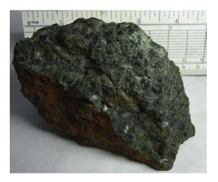
FIGURE 4.29 Dunite is typically coarse grain with light to dark green color rock and consists almost entirely of magnesium rich olivine with minor amount of chromite, pyroxene and pyrope. *Source: Prof. Arijit Ray.*
