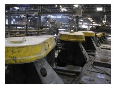
FIGURE 9.18 A typical bank of froth flotation cells in operating circuit to benefit sulfide ore and generate high-grade concentrate.
