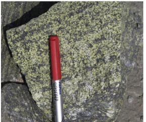
FIGURE 4.31 Dumite, composed of alternate layers of olivine and chromite forming a part of the Sukinda layered Igneous Complex, represent + 90% of chromite resources in India. The group of mines with production capacity of  $\sim 4 \,\mathrm{Mt/a}$  is the second largest in the World after South Africa.
