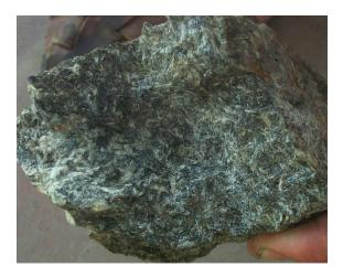
FIGURE 6.5 Quartz-amphibolites or amphibole quartzite is metamorphosed at great depth under high temperature and pressure condition by prograde metamorphism (pictured from Kolihan Section, Khetri copper project, India). The quartz and amphiboles are recognizable in the left and right portions, respectively.
