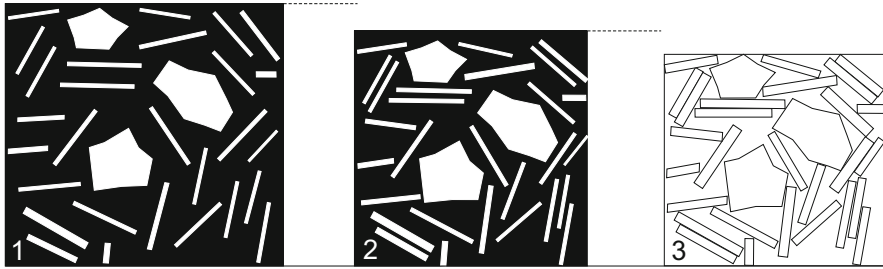
Fig. 4.7 Schematic representation of the drying process of a ceramic mass, for explanations see text. (Modified after Salmang and Scholze 1983)
