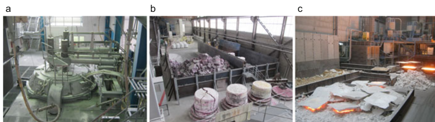
Fig. 9.12 Main operations for the production of synthetic corundum grains: (a) melting of \text{Al}_2\text{O}_3 raw materials in electric arc furnaces at 2000–2100 °C; (b) casting in blocks and cooling; (c) coarse crushing with hydraulic hammers. (Source: Imerys Fused Minerals, Zschornowitz GmbH, with kind permission)
