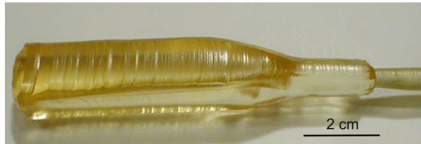
Fig. 8.9 Synthetic piezoelectric single crystal of SNGS ( \text{Sr}_3\text{NbGa}_3\text{Si}_2\text{O}_{14} ) grown from the melt by the Czochralski method
