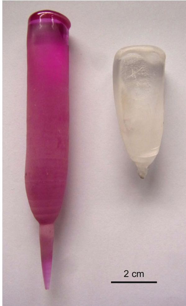
Fig. 10.2 Verneuil fused pears of ruby ( left ) and colorless corundum ( right ) with remnants of the nuclei in the lower part of the aggregates
