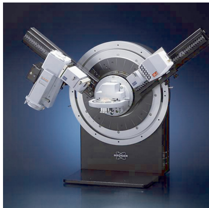
Figure 3.15. Example of an x-ray powder diffractometer manufactured by Bruker AXS. Reproduced with permission of Bruker.
