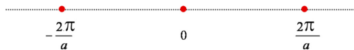
Figure 5.2. One-dimensional reciprocal lattice (red points) spaced 2\pi/a and wave-vectors (black points) spaced 2\pi/L apart.
