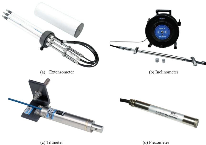
Fig. 4 Instruments used for the ground-based observation in slope stability monitoring
