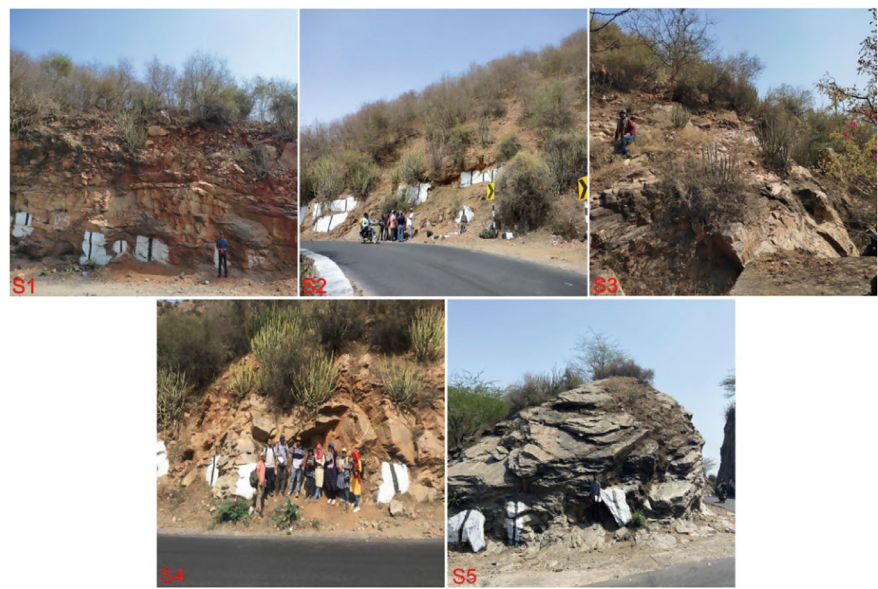
Fig. 4 Field photographs depicting condition of rock mass: (S1) blocky mass prone to rockfall; (S2) soil cover and patchy vegetation on shattered and disintegrated rockmass; (S3) failed blocky mass along cut slope; (S4) adversely oriented discontinuities forming Planar failure and few wedges; (S5) discontinuity sets prone to Planar as well as wedge failure
