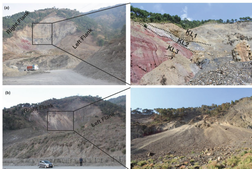
Fig. 3 a Field photograph of showing critically stable right flank during year 2018 field visit and b field photograph of showing failed right flank during year 2022 field visit
