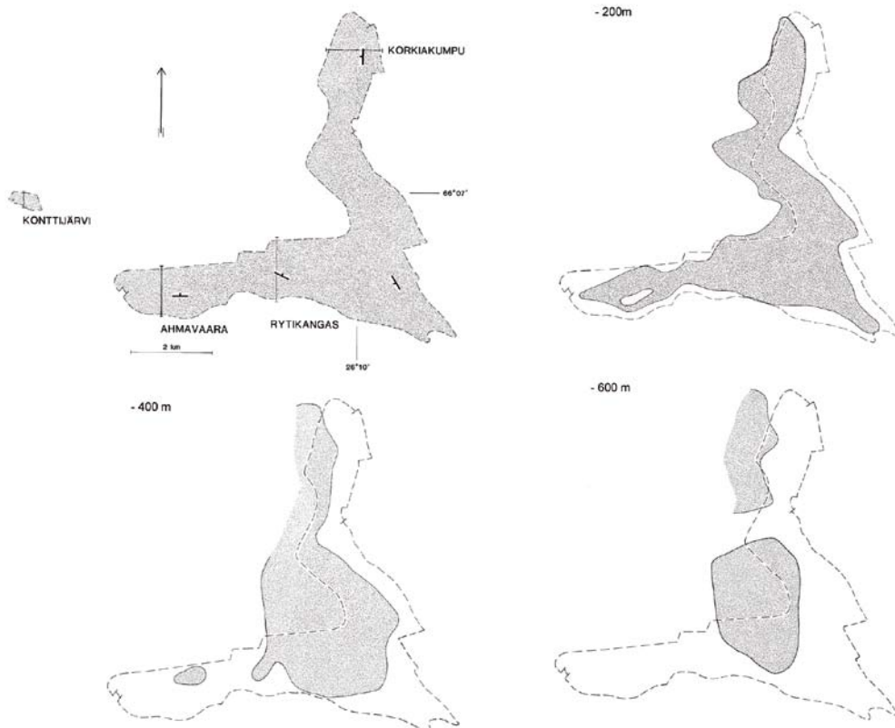
7. Suhanko Intrusion: plan view and horizontal cross-sections at depths of 200, 400 and 600 metres. Sites of the vertical cross-sections depicted in Figure 8 are also shown. Modified after Pernu et al. (1986).
