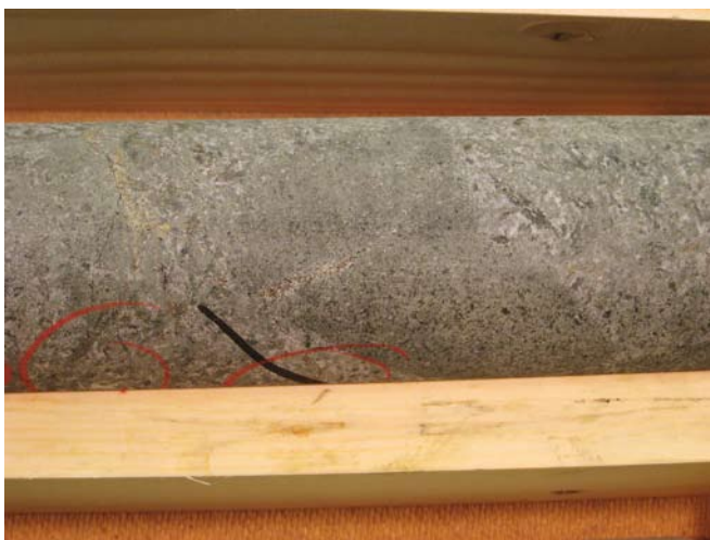
4. A, Fine-grained and sharp-edged chill margin fragments in the Ahmavaara drill core. For structural position see Figure 6. B, cresscumulate with sulphides in the lower part of the Ahmavaara marginal series.
