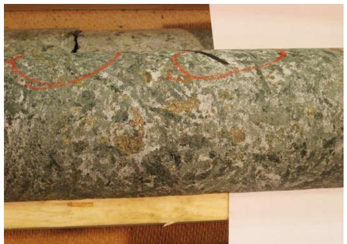
4. A, Fine-grained and sharp-edged chill margin fragments in the Ahmavaara drill core. For structural position see Figure 6. B, cresscumulate with sulphides in the lower part of the Ahmavaara marginal series.
