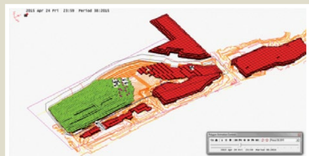
Figure 2: Deswik simulation of terrace mining at Dawson (green is spoil to be moved and red is spoil that has been moved).
