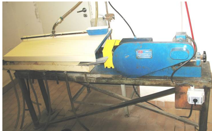
Fig. 6.7. Concentrating table (top view) (a) and a photograph (b)
