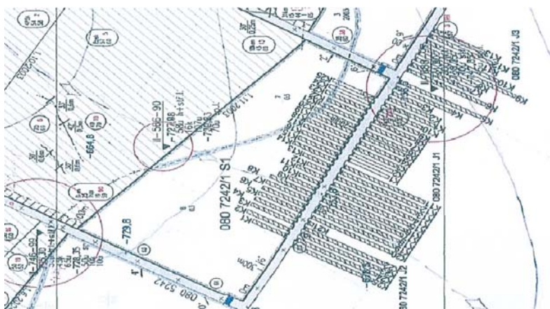
Figure 9. Section of seam map with marked holes drilled by the auger machine VS-SEAL-625 P1 (source: Kosnovsky 2008).
