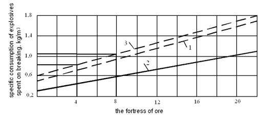
Figure 2. Change of specific consumption of explosives depending on ore hardness: 1 – well diameter 85 mm; 2 – well diameter 65 mm; 3 – well diameter 100 mm.
