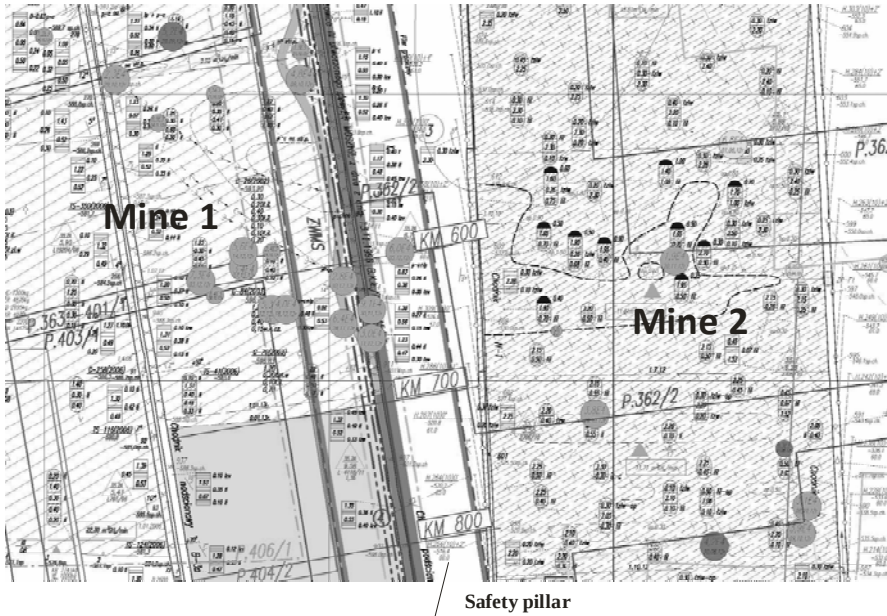
Figure 3. Increased seismic activity due to superposition of impact manifested by zones of increased stress.
