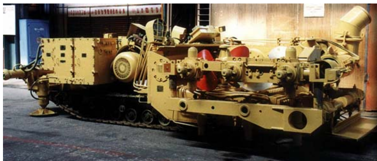
Figure 5. Coal augering machine type BZM-1M1 produced by Morozov company from Charkov, Ukraine (source: www.morozov.com.ua ).
