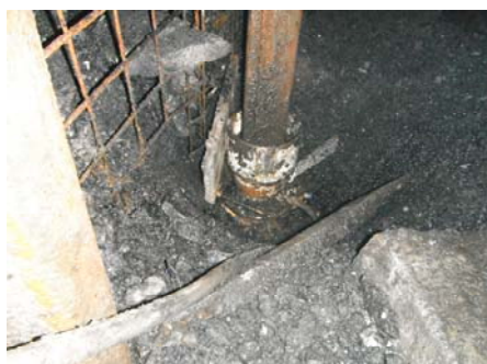
Figure 11. ŁPw mining supports installed in the riser 3 research on board the 504 in coal mine “Bobrek-Centrum” (Kuziak 2012).
