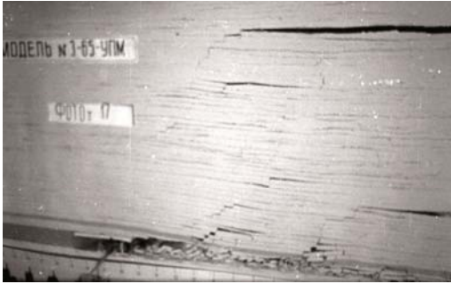
Figure 2. Rocks dislocation model during C_5 coal seam mining.
