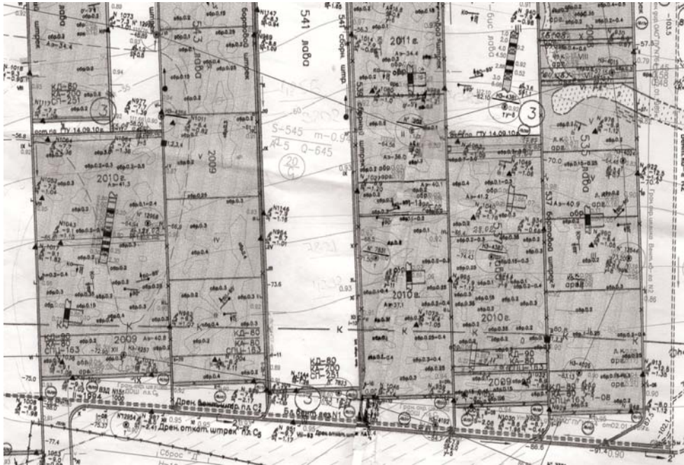
Figure 1. Plan of mining operations of C_5 with an indication of places of the complex subsidence on rigid base.
