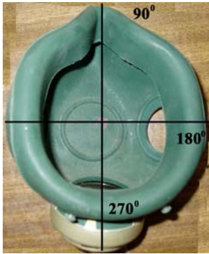
Figure 4. Axisymmetric distribution of mechanical pressure along obturation bar.
