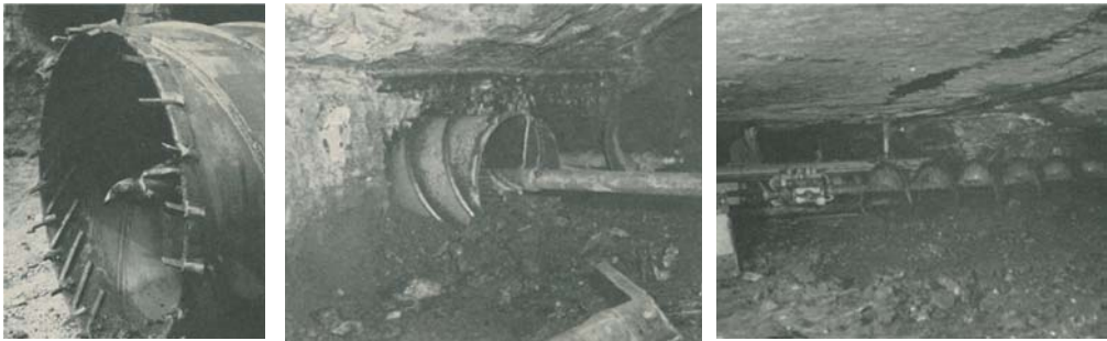
Figure 2. Augering machine Cardox-Hardsocg during exploitation of Elkhorn seam at Pike County (source: Newell and Storey 1952).
