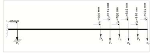
Figure 2. Scheme of the lever of the second kind for load compensation.
