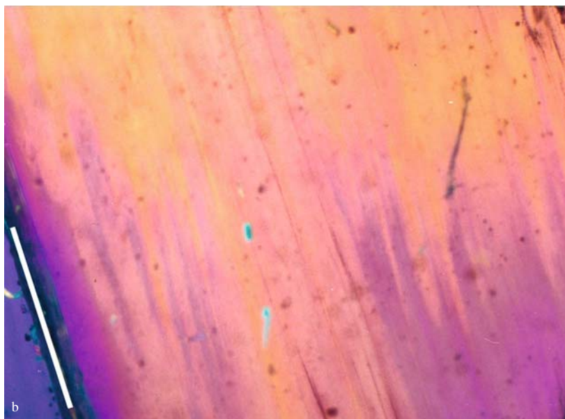
Figure 3.8. (a) Subsector zoning in alum (K_{0.77}Rb_{0.23})Al(SO_4)_2 \cdot 12H_2O {111}, section parallel to (111) growth face. Sub-sector boundaries shown by bold lines are the boundaries between different vicinal faces on the crystal surface. Sub-sector boundaries shown by thin lines are observed between crossed polarizers. Numbers denote birefringence \times 10^{-7} . (b) The same crystal with section through the center of (111) face parallel to the growth direction [111] between crossed polarizers and with a first order red retarder. White line marks position of (111) face
