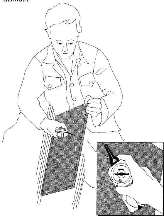
Fig. 19. The contact method of measuring strike.
