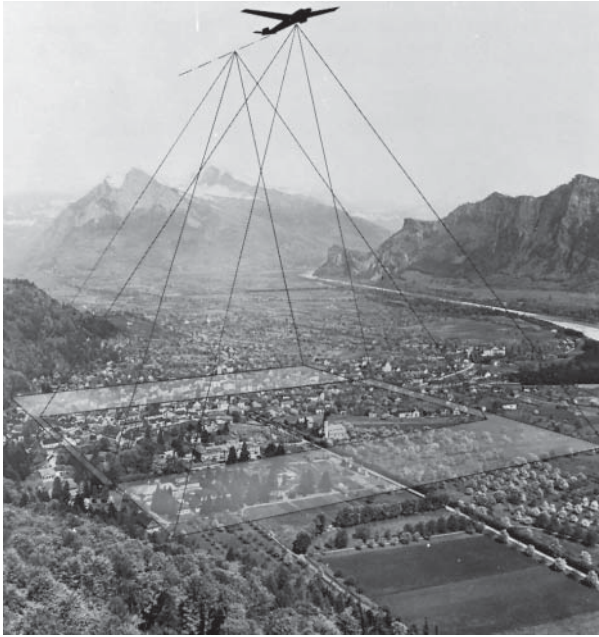
Figure 3.3 Acquisition of successive photographs yielding a stereopair. (Courtesy Leica Geosystems.)
