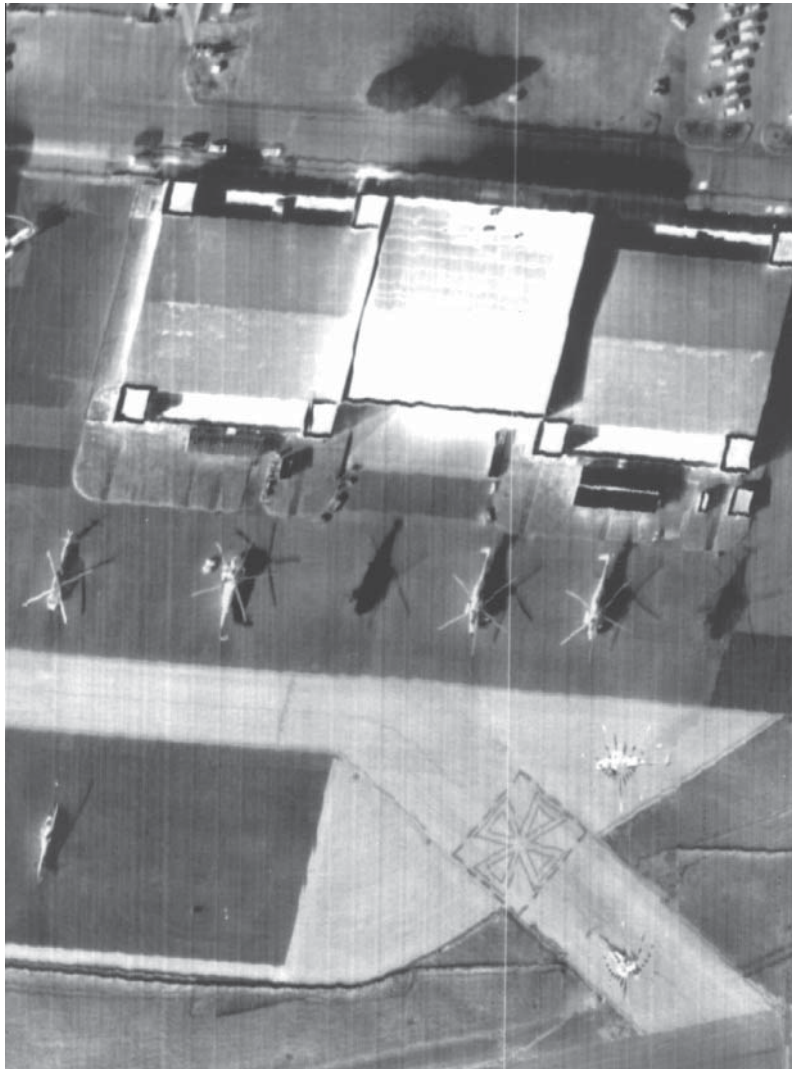
Figure 4.31 Daytime thermal image, Quantico, VA, 0.25 mrad IFOV. (Courtesy Goodrich ISR Systems.)
