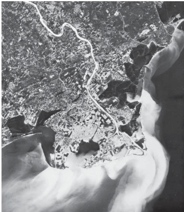
Figure 8.16 Space photograph (taken with the Large Format Camera) showing the silt-laden Po River discharging its sediments into the Adriatic Sea. Scale 1:610,000. (Courtesy NASA and ITEK Optical Systems.)
