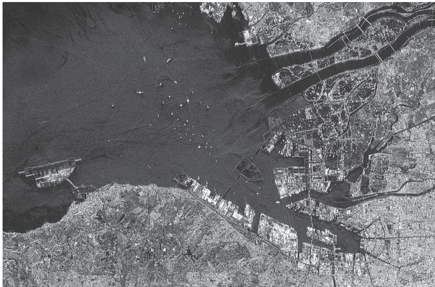
Figure 6.45 ALOS PALSAR image of Nagoya, Japan, April. Scale 1:315,000. Black-and-white copy of a color multipolarization L-band image. (Courtesy NASDA.)
