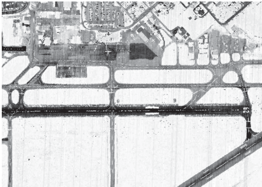
Figure 6.66 Lidar intensity image of a portion of the Lewiston/Nez Perce County Airport, Idaho. The data were acquired by a Leica Geosystems ALS 40 Airborne Laser Scanner at 24,000 pulses per second and 2-m post spacing. (Courtesy of i-TEN Associates.)
