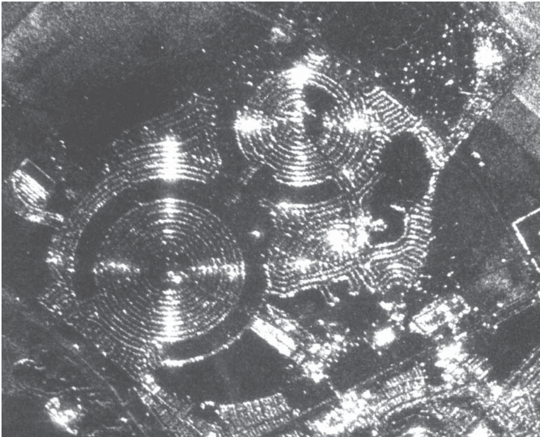
Figure 6.37 Airborne SAR image, Sun City, AZ, X band. The look direction is from the top of the image. Scale 1:28,000. (From American Society for Photogrammetry and Remote Sensing, 1998. Images copyright © John Wiley & Sons, Inc.)
