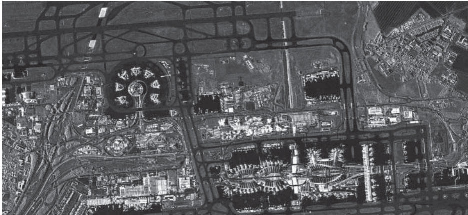
Figure 6.49 Charles de Gaulle Airport, France, shown in a TerraSAR-X High Resolution Spotlight image (scale 1:67,000). Full resolution of this image is 2.4 m. (Copyright: DLR e.V. 2009, Distribution Airbus DS/Infoterra GmbH.)
