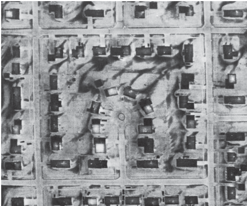
Figure 4.33 Nighttime thermal image depicting building heat loss in an Iowa City, approximately 2:00 A.M., snow-covered ground, air temperature approximately -4^{\circ}\text{C} , 460 m flying height, 1 mrad IFOV. (Courtesy Iowa Utility Association.)
