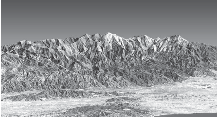
Figure 6.52 Perspective view of a DEM of the Los Angeles area, derived from SRTM interferometric radar data. A Landsat-7 ETM+ image has been draped over the DEM to show land cover patterns. (Courtesy NASA/JPL/Caltech.)
