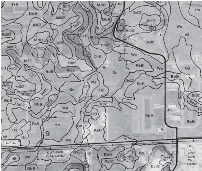
Figure 8.4 Portion of a USDA–ASCS soil map, Dane County, WI. Original scale 1:15,840 (4 in. = 1 mile). Printed here at a scale of 1:20,000. (Courtesy USDA-ASCS.)
