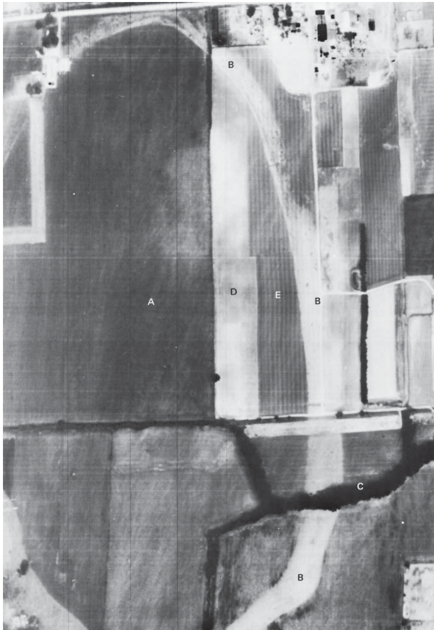
Figure 4.29 Daytime thermal image. Middleton, WI, 9:40 A.M., 600 m flying height, 5 mrad IFOV. (Courtesy National Center for Atmospheric Research.)
