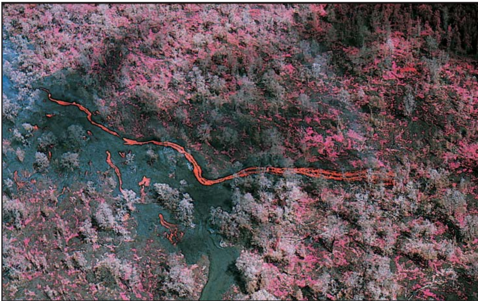
Plate 5 Oblique normal color (a) and color infrared (b) aerial photographs showing flowing lava on the flank of Kilauea Volcano, Hawaii. The orange tones on the color infrared photograph represent infrared energy emitted from the flowing lava. The pink tones represent sunlight reflected from the living vegetation. (Author-prepared figure.) (For major discussion, see Section 2.4.)
