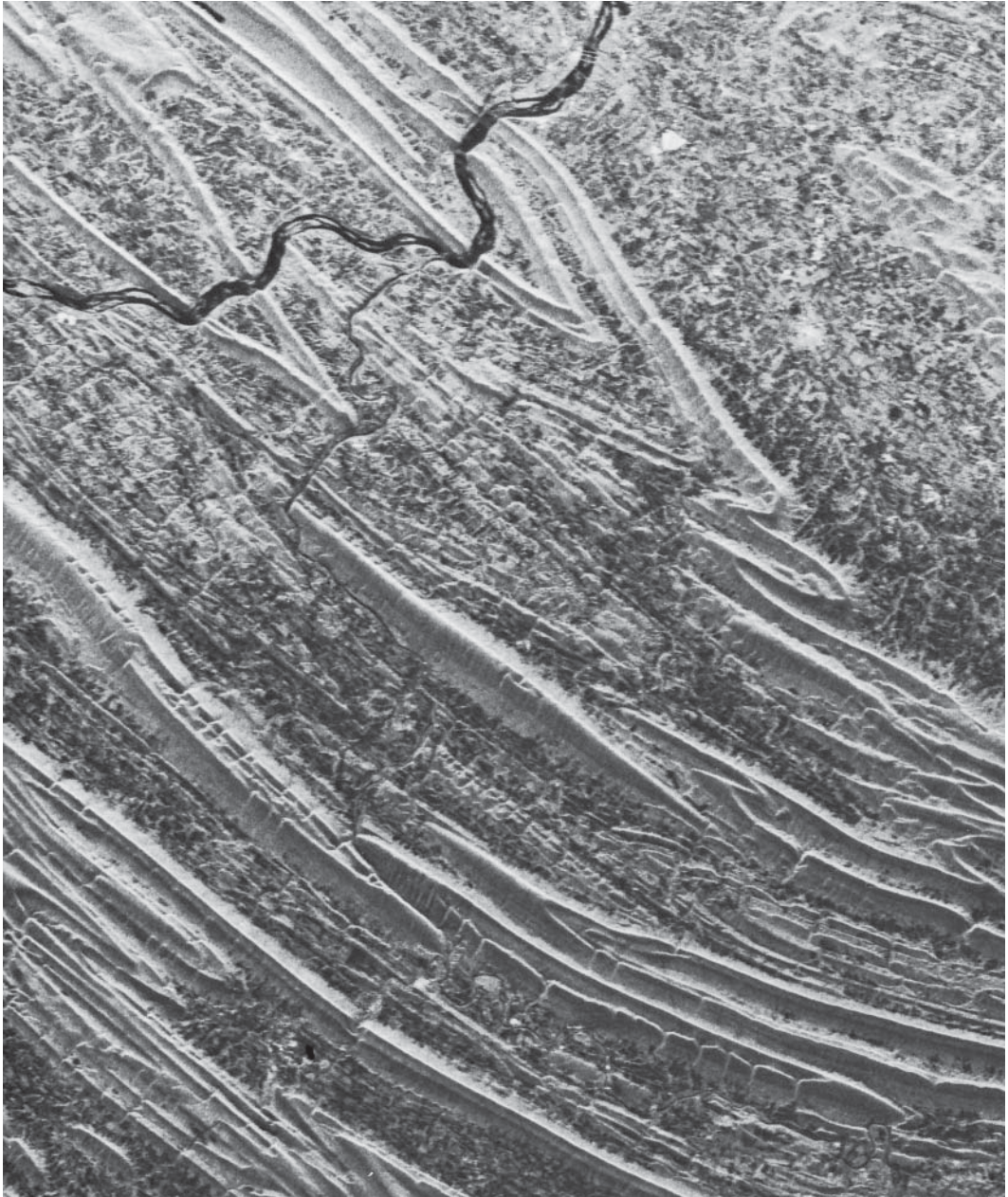
Figure 6.5 Seasat radar image of Appalachian Mountains of Pennsylvania, L band, midsummer. Scale 1:575,000. (Courtesy NASA/JPL/Caltech.)
