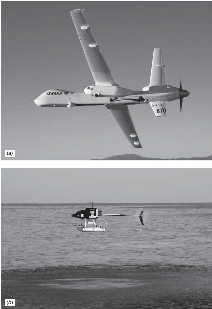
Figure 1.24 Uninhabited aerial vehicles (UAVs) used for environmental applications of remote sensing. (a) NASA's Ikhana UAV, with imaging sensor in pod under left wing. (Photo courtesy NASA Dryden Flight Research Center and Jim Ross.) (b) A vertical takeoff UAV mapping seagrass and coral reef environments in Florida. (Photo courtesy Rick Holasek and NovaSol.)
