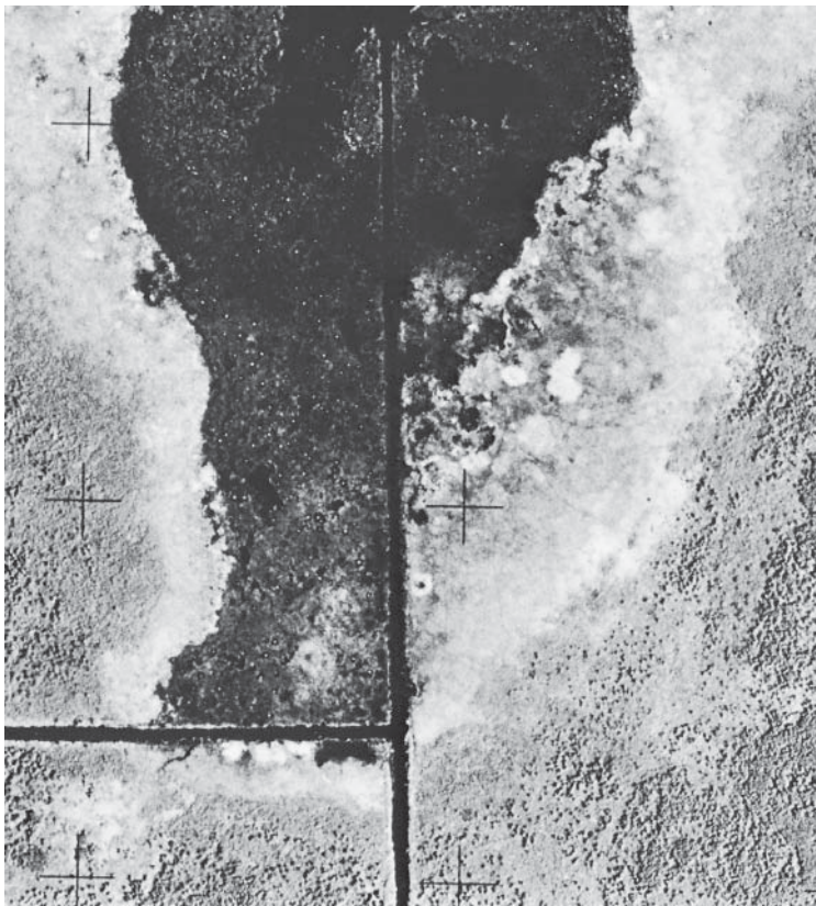
Figure 8.20 Black-and-white copy of a color infrared aerial photograph of Sheboygan Marsh, WI. Scale 1:13,000 (enlarged 4.6 times from 1:60,000). Grid ticks appearing in image are from a reseau grid included in camera focal plane. (Courtesy NASA.)
