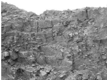
Figure 3.1 Rock mass with several discontinuities.
