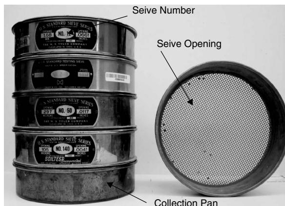
FIGURE 1.12. Stack of sieves used for grain size analysis.
