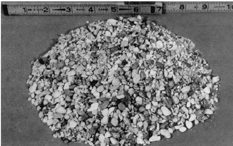
FIGURE 1.17. Poorly graded soil (from [14]).
