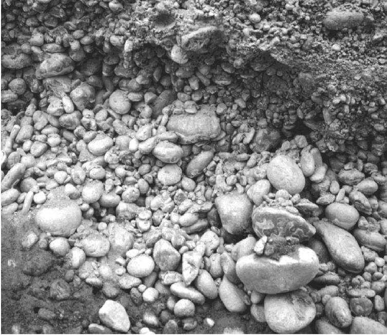
**FIGURE 3.5.** Very well sorted (poorly graded) coarse gravel deposited near Hanford, Washington during an enormous flood associated with the last ice age.
