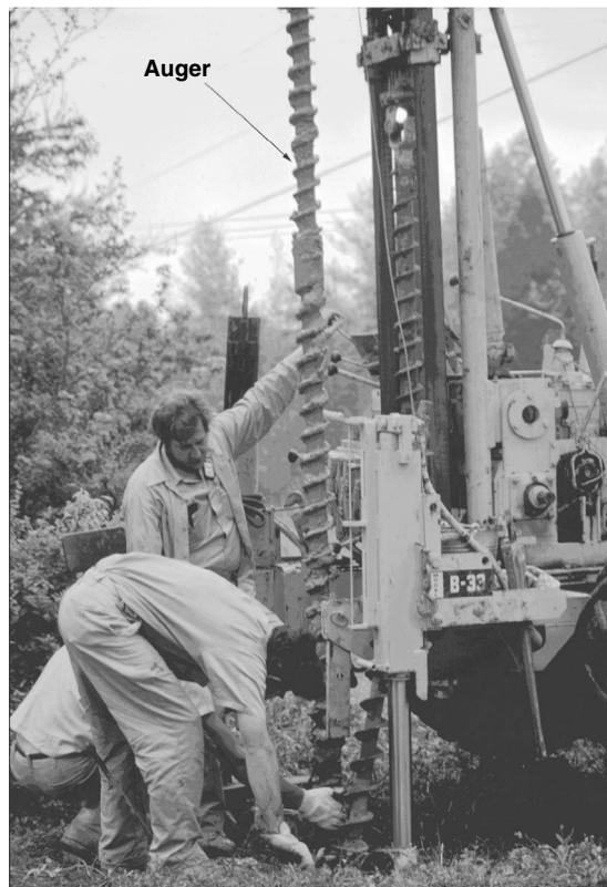
FIGURE 3.42. Truck-mounted auger.
