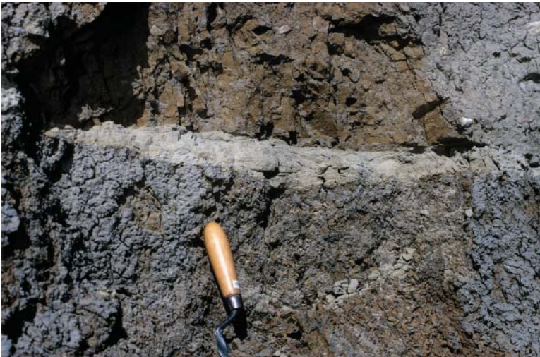
Figure 11.7 Example of a sub-till stratified lens lying beneath a thin ice stream bed till and overlying relatively impermeable substrate of shale in Alberta, Canada.
