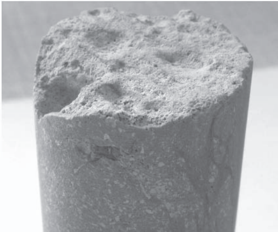
Figure 6. Inlet end of the Weyburn reservoir rock sample after the CO 2 flooding experiment carried out at GEUS. Numerous small pits are present in the sample surface after the experiment. They represent dissolved calcite grains. (Riding and Rochelle, 2005; photograph reproduced with kind permission of GEUS).
