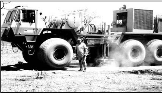
Fig. 5-47 Side View of a Truck-mounted Vibrator
