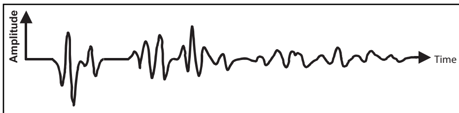
Fig. 3-16 Noise-free Seismic Trace Derived from Earth Reflectivity Function
