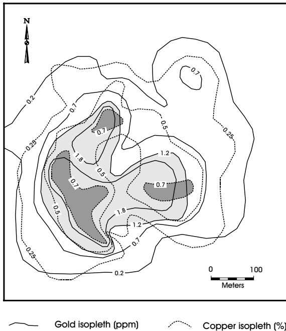
Figure 2.19: Metal distribution patterns in the Dizon deposit, Philippines. Solid contours are for Au (g/t); dotted contours are for Cu (%). The 1.2 g/t Au contour delineates a zone characterized by both high-gold and high-copper grades. After Sillitoe (1993).
