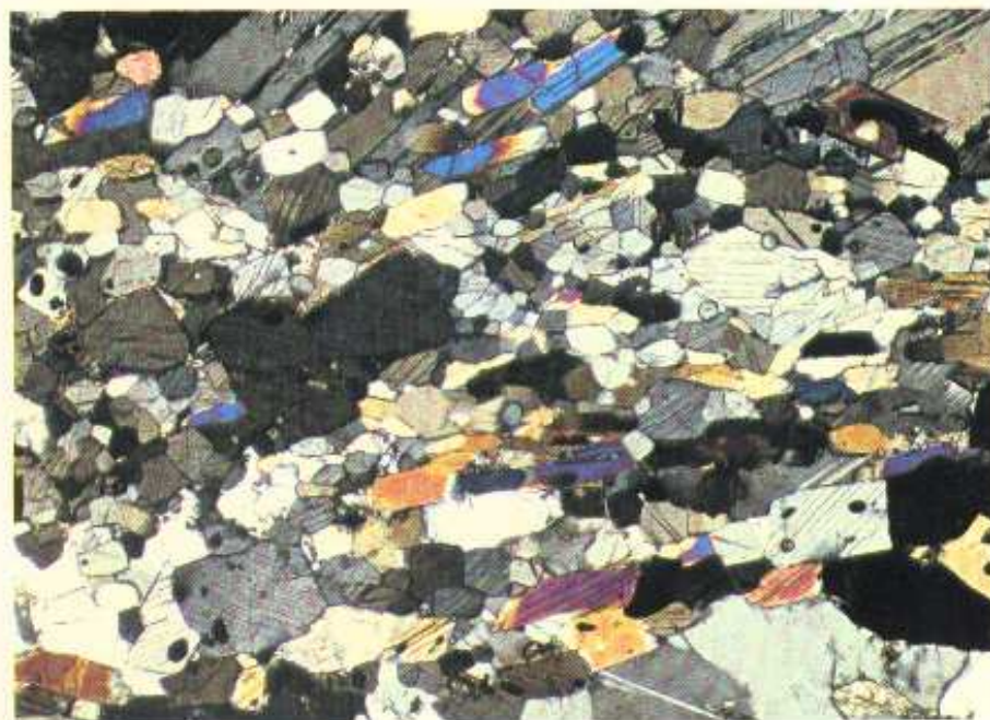
Specimen from garnet–cordierite–sillimanite gneiss, Ithoty, Madagascar; magnification \times 40 .
