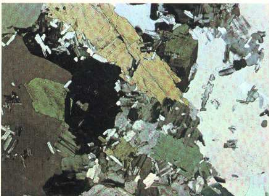
Specimen from syenite, Himaussaq intrusion, West Greenland, magnification × 32.
