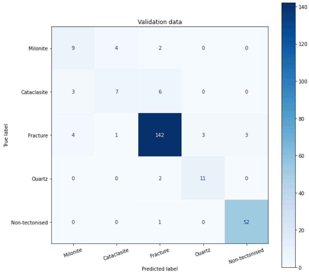
Figure 38. A confusion matrix for the ResNet-101-based GTD-2 interpretation algorithm inference on a validation dataset.
