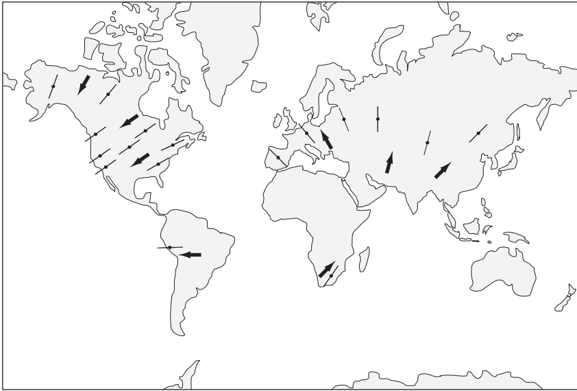
FIGURE 4.10 Fast S-wave velocity directions in the subcontinental lithosphere compared to motion directions of modern plates (bold arrows). After Silver & Chan (1991).
