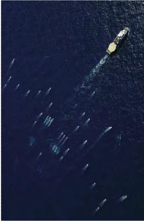
Figure 7 Aerial view of an offshore seismic survey, showing the array of hydrophones being towed behind the ship. Reproduced with permission of Millenium Atlas Company Limited.
