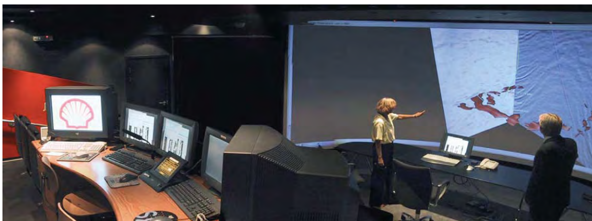
Figure 14 Three dimensional seismic interpretation system (so called ‘visionarium’).
