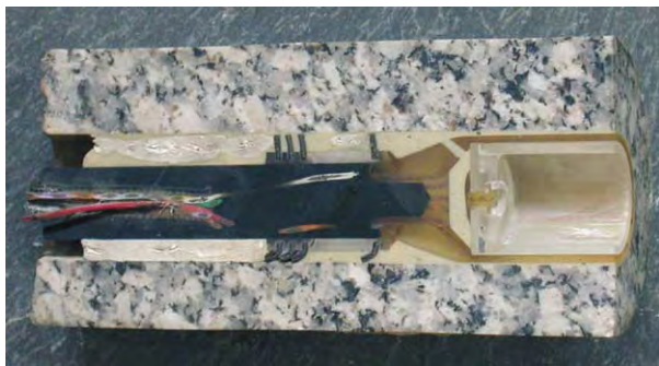
Figure 2 An overcoring device for stress estimation, sectioned after recovery from the test borehole. The control wires enter at the left; the part of the cell carrying the strain gauges, and which is cemented into the borehole, is at the right.
