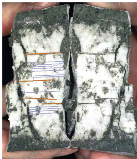
Figure 3 Core sample number 1249F 8h 2, from the Ocean Drilling Program Leg 204, drilling on Hydrate Ridge, the Cascadia Accretionary Prism, off the coast of Oregon, USA. The sample shows how gas hydrates (white) may occur in shallow, porous sediments. Photograph courtesy of Anne M Tréhu and the Shipboard Scientific Party, Ocean Drilling Program Leg 204, 2003.
