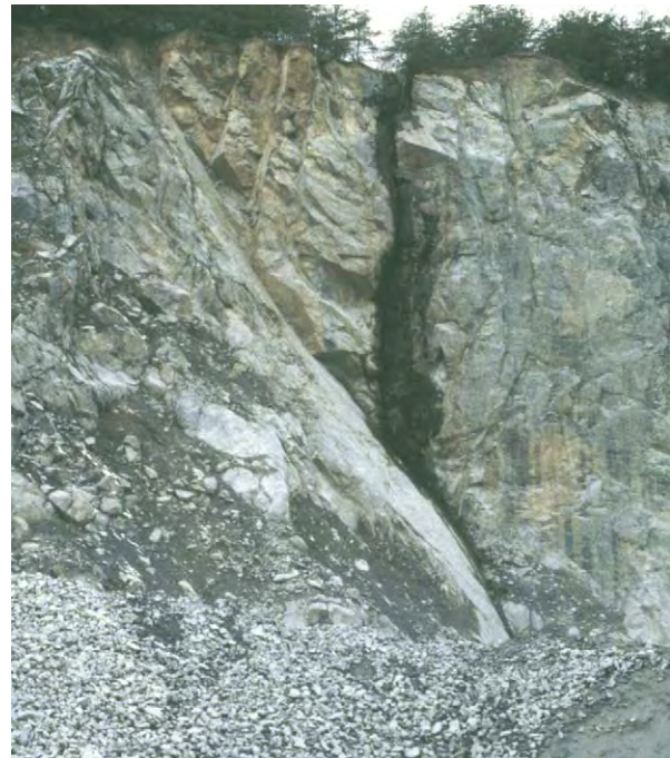
Figure 1 Quarry operated for construction aggregate, road metal, and granular fill, in dolerite (diabase) and high grade crystalline metamorphic country rock of Prince George’s County, Maryland, USA; the vertical face is approximately 15 m high. The pit has reached the lateral limits of the deposit of usable rock and also has come to the maximum viable depth for maintenance of the pit, removal of groundwater seepage, and precipitation runoff. The site was being considered for conversion to a long term secondary use compatible with environmental protection requirements. Photograph by the author.
