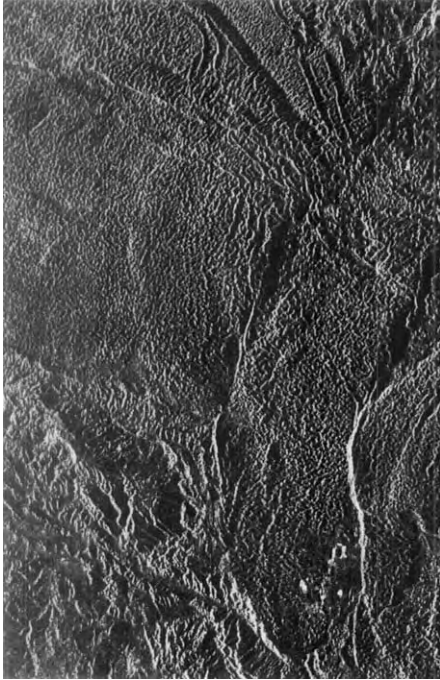
Figure 2 Radar amplitude image of part of north central Jamaica viewed by the SEASAT L band radar in 1978. The radar illumination is from the left (west south west) of the image at an incidence angle of about 20 degrees from vertical. Most of the scene is covered by "dimpled" pattern typical of tropical karst topography of Cenozoic limestones, except for the bottom left corner which is an inlier of Cretaceous volcanic and volcanoclastic rocks. In the northernmost central part of the image a straight normal fault scarp downthrows the limestones to the north. This is cut by one of two, subparallel curving fault scarps. The easternmost one shows the clear pattern of a scissor fault. To the south the fault shows a west facing escarpment that is bright in the image and further north this changes to an east facing escarpment in shadow. The image measures about 36 \times 24 km.
