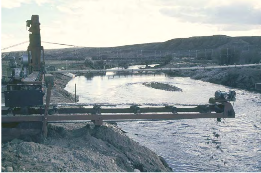
Figure 4 A field facility for bedload sampling and measurement installed by the United States Geological Survey on the East Fork River, Wyoming.
