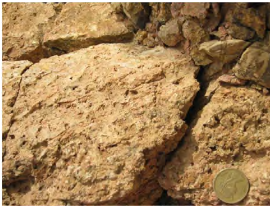
Fig. 1.6. Episyenite (quartz dissolution of granite leaving cavities).
