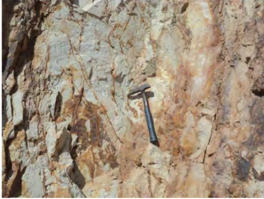
Fig. 1.9. Joints in microgranite stained by iron oxides.
