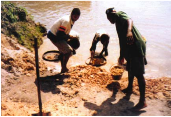
Fig. 95 Screening of diamond-bearing gravel by artisanal miners in the Kerouane region.
