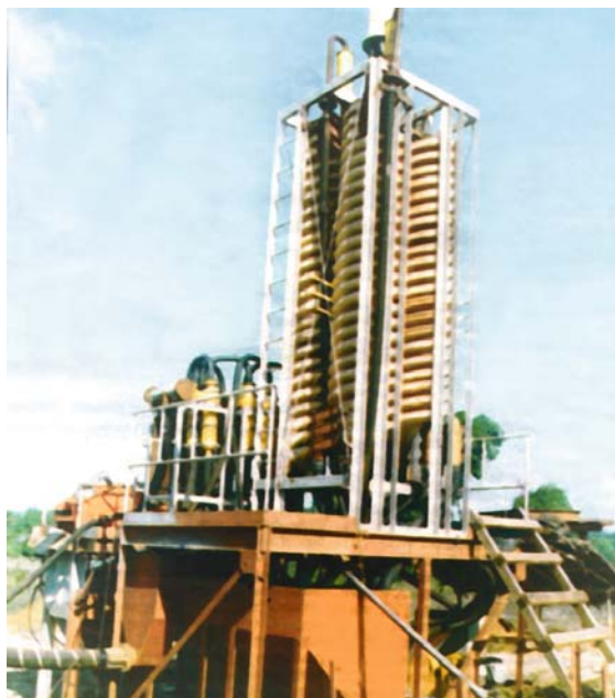
Fig. 103 Machinery to be used for the production of ilmenite, rutile and zircon from beach sands at Kwale.
