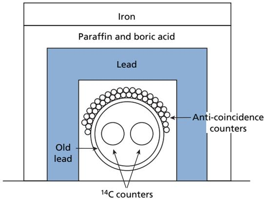
**Figure 4.6** Libby's anti-coincidence counting. Geiger counters whose gas contains the  $^{14}\text{C}$  to be measured are surrounded by a series of layers of shielding as protection from cosmic rays (only old lead is used so that the uranium chains are dead and there is no decay from them). When the small counters record a disintegration, it is due to cosmic radiation and so is subtracted from the value recorded by the central counter.
