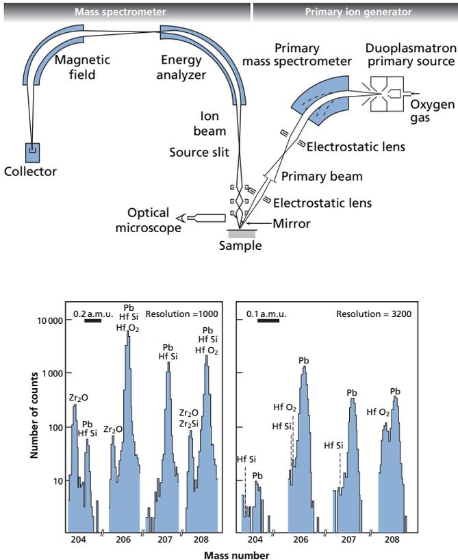
**Figure 3.31** An ionic probe and mass spectra. Top: diagram of an ionic probe. Bottom: mass spectra obtained at resolutions of 1000 and then 3200. The solution to the problem of isobaric interference can be seen. Plate 3 (top) also shows an ion probe.
