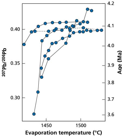
Figure 3.13 The  $^{207}\text{Pb}$ – $^{206}\text{Pb}$  spectrum obtained by thermo-ionization of lead. This spectrum is obtained by progressively heating the filament after having deposited zircon on it. The example shown is of detrital zircon from Australia, among the oldest recorded (Kober, 1986).
