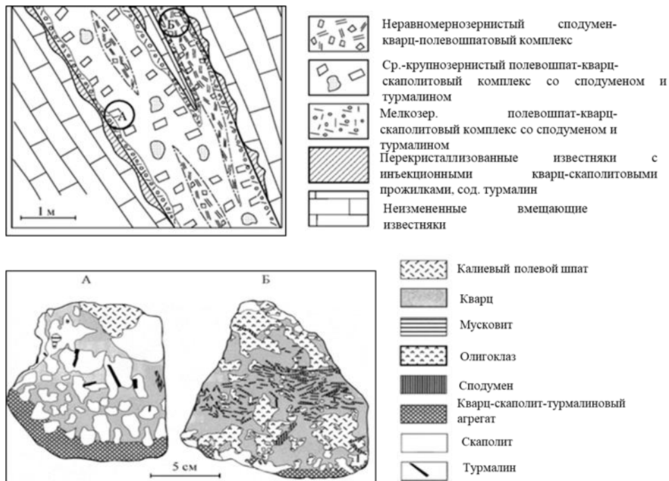
Figure 4. Geological structure of the pegmatite vein (in Russian).
