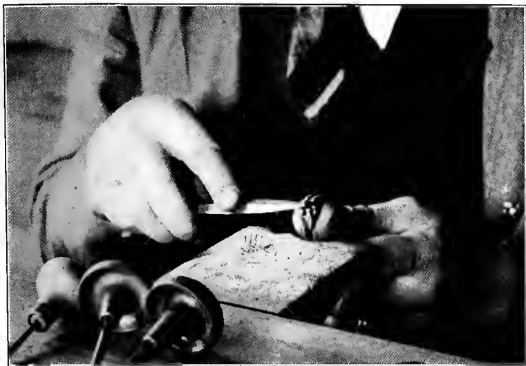
FIGURE 96. Filing the top of prongs
