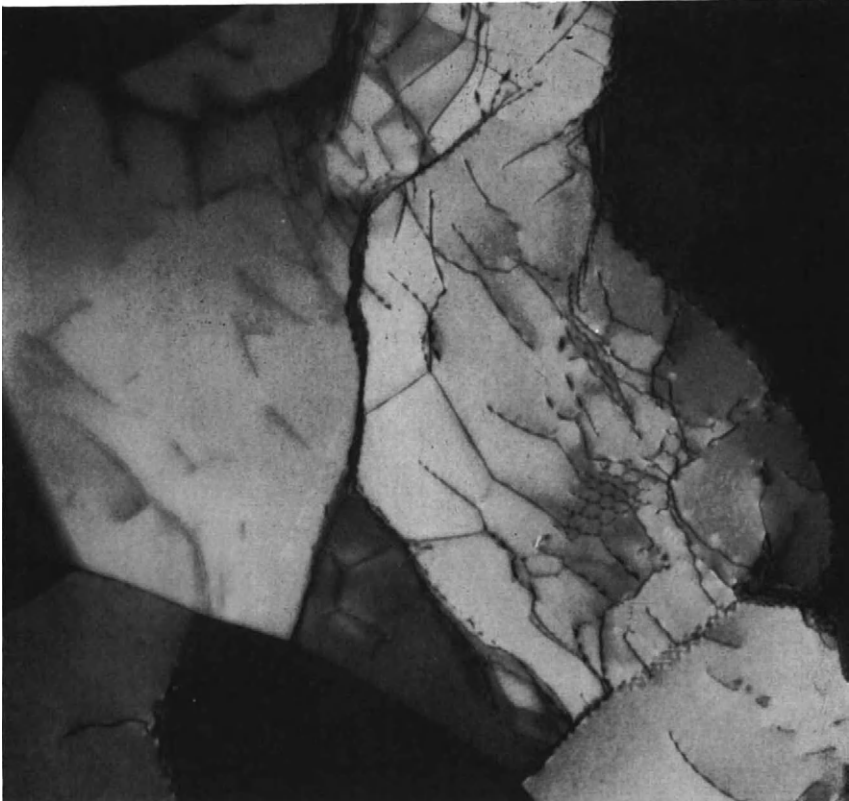
PLATE V. (a) Cell structure in rolled chromium sheet. Cells are 2 to 4\mu across and are bounded by dislocation tangles. (b) Annealing of (a) produces sub-grain boundaries mainly of hexagonal dislocation networks (electron photomicrographs from McLaren, 1964)
