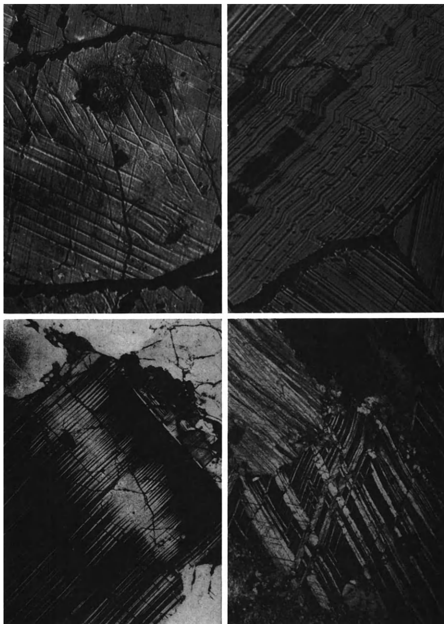
PLATE XI. (a) Two sets of (110) slip lines on experimentally deformed olivine (Raleigh, 1964). (b) Traces of (100) slip lines in kyanite. Kink bands with external rotation about [010] (Raleigh, 1964). (c) Deformation twins in plagioclase from charnockite ( \times 25 ). (d) Conjugate deformation twins in calcite from marble ( \times 15 )
