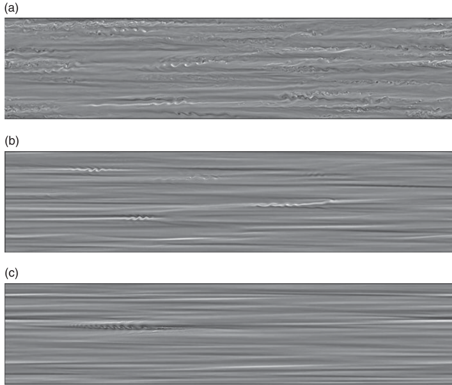
Figure 8.8. Vertical ( x,z ) slices of the y component of vorticity in simulations with fixed \nu = 0.03125 \text{ cm}^2/\text{s} and different N (and hence different Fr_h and Re_b ), corresponding to Re_b = 2.6 (top), 0.69 (middle), and 0.18 (bottom) (runs A6, B6, and C6). Shading is saturated to white/black at \pm 3 \text{ s}^{-1} . Fields in (a) and (b) are plotted at the final time of the simulations t = 2000 \text{ s} . Panel (c) is plotted at t = 1900 \text{ s} , which was chosen to illustrate the lone patch of Kelvin-Helmholtz billows visible at this time.
