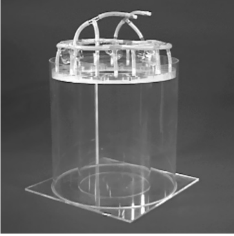
Figure 9.2. Cylindrical annulus used for the QBO experiments conducted at the University of Kyoto as part of the GFD-Dennou Club. Used with permission, Sakai [1997] and Otobe et al. [1998]. The oscillating membrane can be seen at the top of the annulus, while in the original experiment of Plumb and McEwan the membrane was mounted at the bottom.
